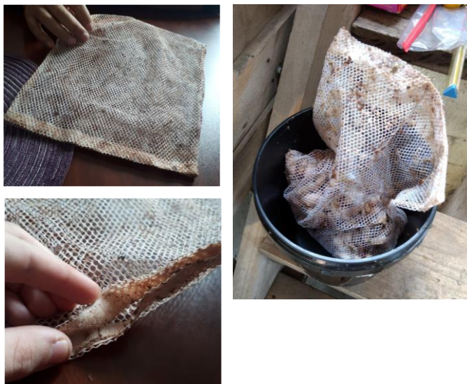
Figure III.1 Pictures of the mesh bags used for the 1 kg subsamples in the fermentation experiments. Top left, empty mesh bag. Bottom left, mesh bag Velcro closing. Right, mesh bag with 1 kg subsample, sampled after one day of fermentation.
