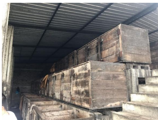
Figure III.2 Picture of a cascade fermentation setup, similar to the setup used in the fermentation experiments for batches A and B.
