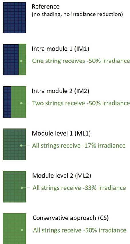
Figure 12: Generic cases used to illustrate how shading can be implemented in BIPV models.
