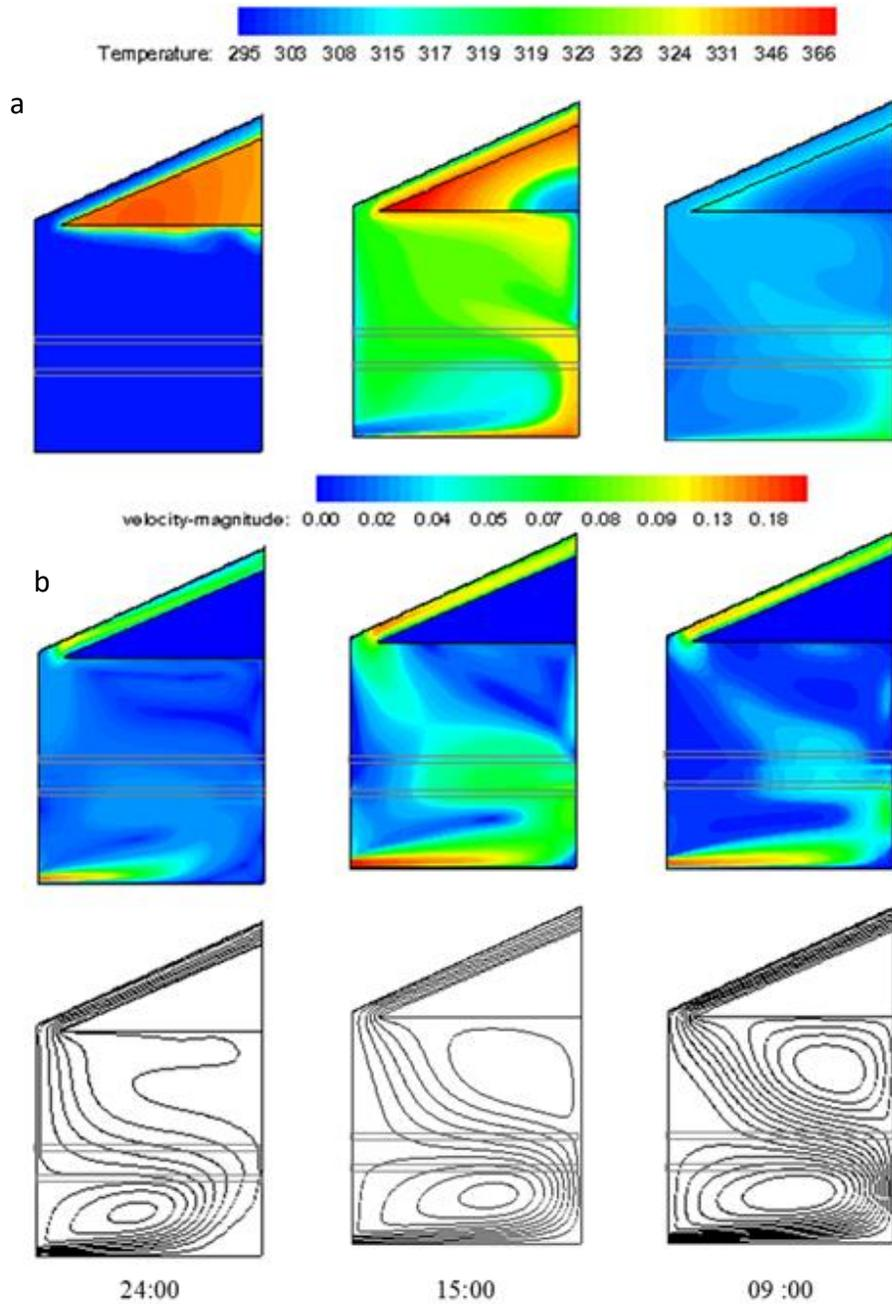
Figure 19: Temperature (a) and velocity distribution (b) of solar fig dryer using CFD (Khaldi et al., 2018).
