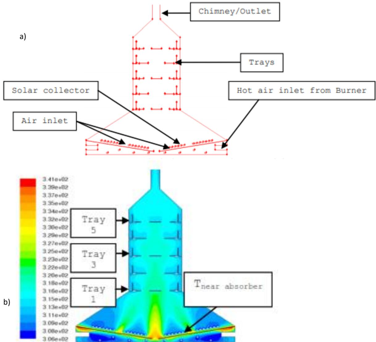
Figure 8: Solar cabinet dryer model (a) and temperature contours (b) in degree centigrade, (Yunus and Al-Kayiem, 2013).
