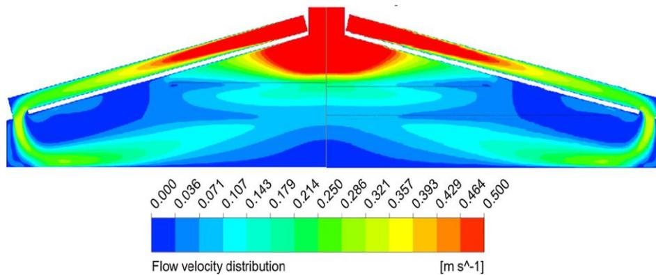
Figure 16. Contour plot of velocity distribution of the solar sweet potato drying cabinet (Tegenaw et al., 2019b)
