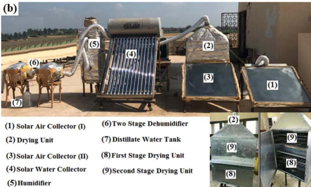
Figure 4: A two-stage indirect solar dryer with rearming coupled with humidification-dehumidification, (a) schematic diagram and (b) photo (Kabeel and Abdelgaied, 2018)
