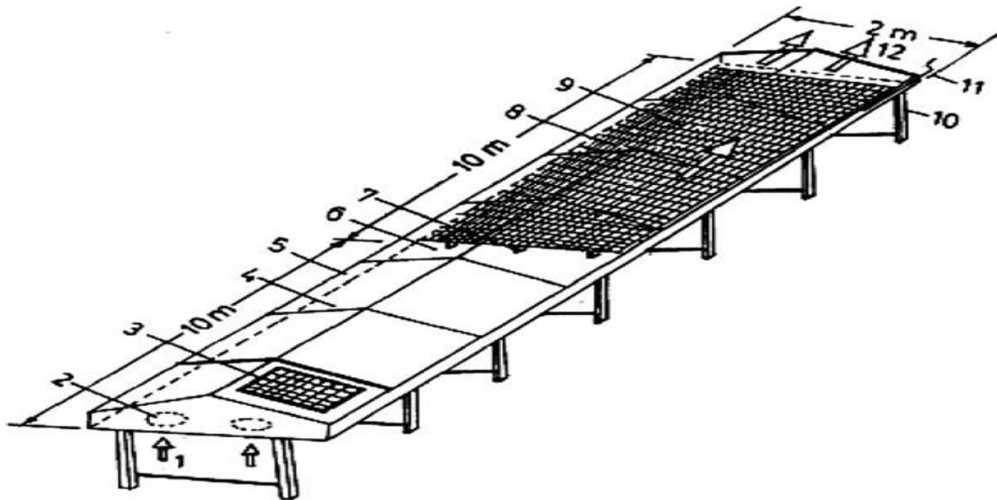
Figure 5: Solar tunnel drier: 1. air inlet; 2. fan; 3. solar module; 4. solar collector; 5. side metal frame; 6. outlet of the collector; 7. wooden support; 8. plastic net; 9. roof structure for supporting the plastic cover; 10. base structure for supporting the drier; 11. rolling bar; 12. outlet of the drying tunnel (Hossain and Bala, 2007).
