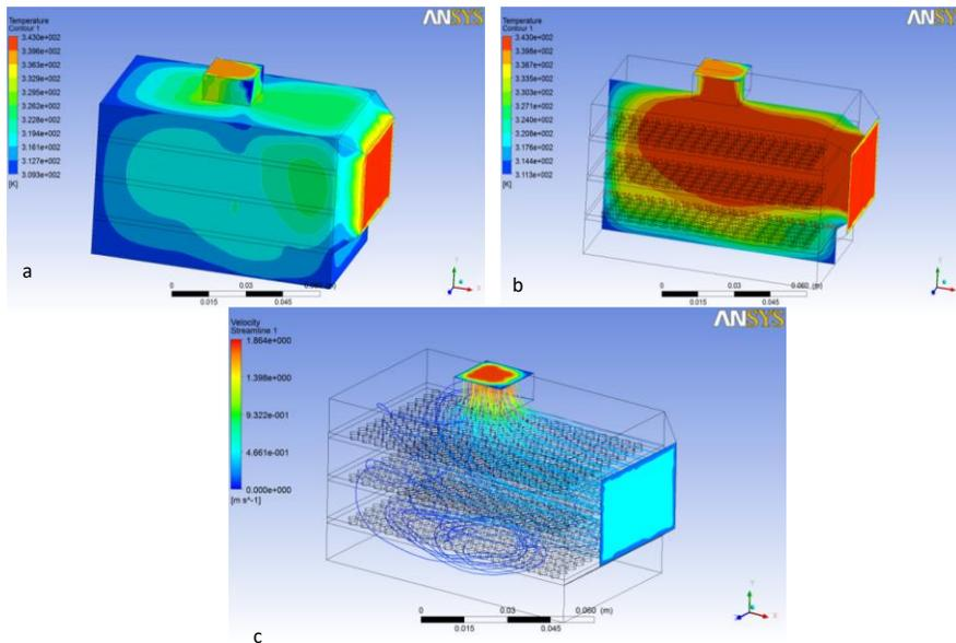
Figure 12. Temperature contours (a) the wall (b) midplane and (c) velocity streamlines of the cabinet dryer at 14:00 for airflow rate of 0.025 kg/s (Iranmanesh et al., 2020).
