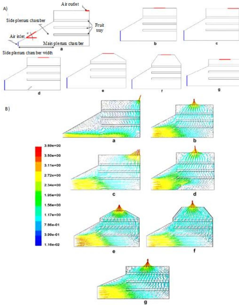
Figure: 7. Air velocity distribution profiles for the seven designs (A) and CFD simulation results (B) at inlet air velocity =  $3 \text{ m s}^{-1}$  (Amanlou and Zomorodian, 2010).
