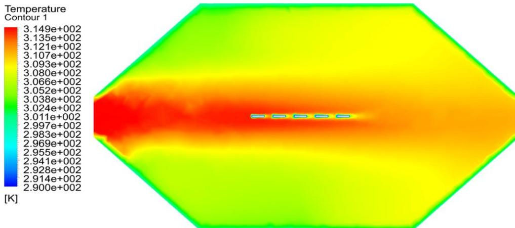
Figure14. Temperature distribution in the drying chamber (Güler et al. 2020).
