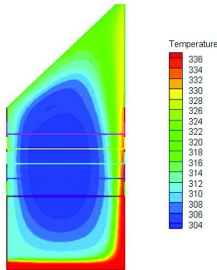
Figure 17: Temperature contour of the drying chamber in kelvin (Ghaffari and Mehdipour, 2015).
