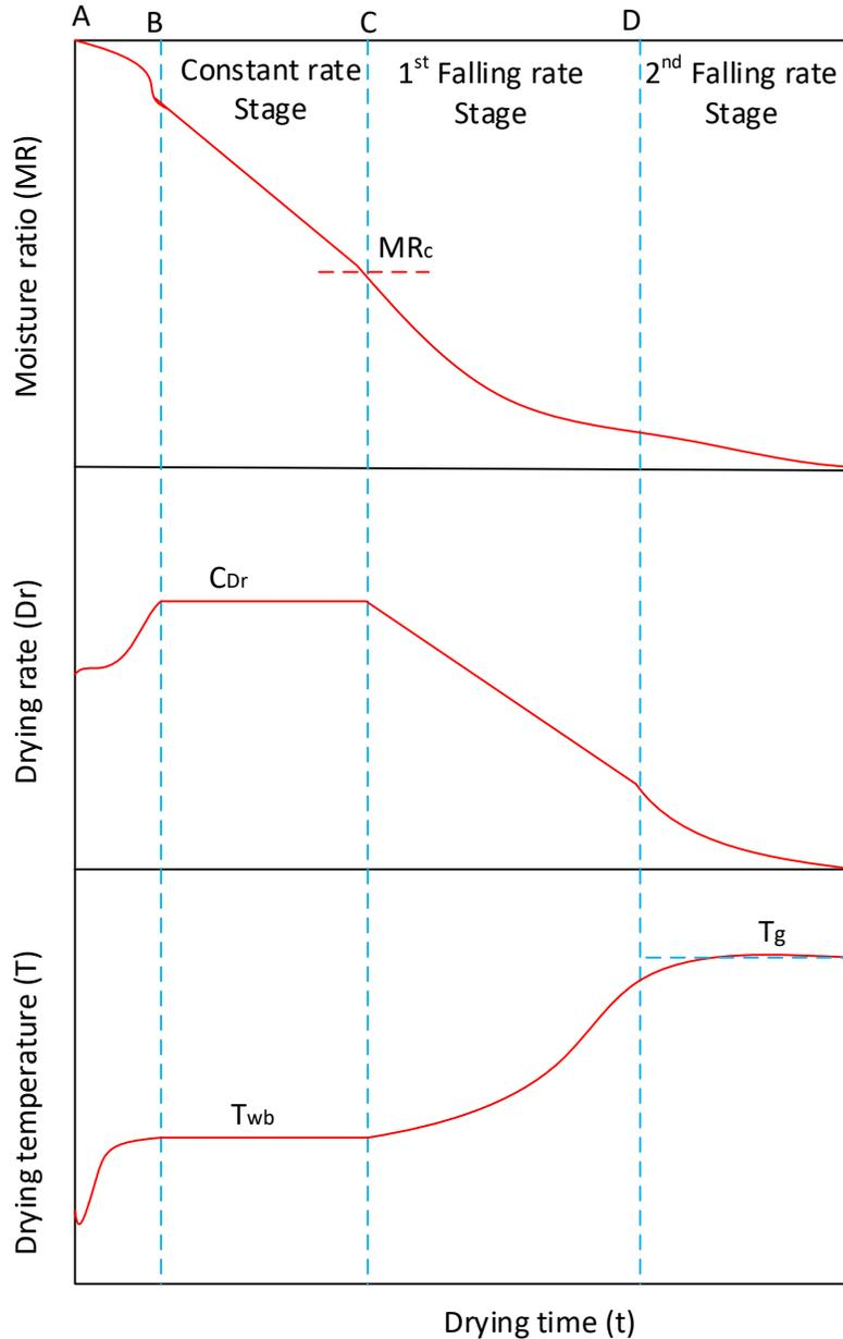
Figure 1: Drying curve of agricultural products that shows constant rate and falling rate periods. (Onwude et al., 2016)
