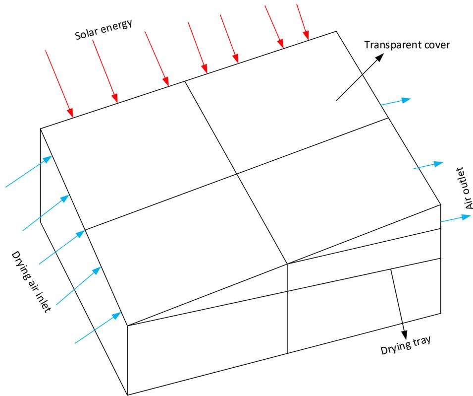
Figure 2: Direct solar dryer (Kumar et al., 2016).
