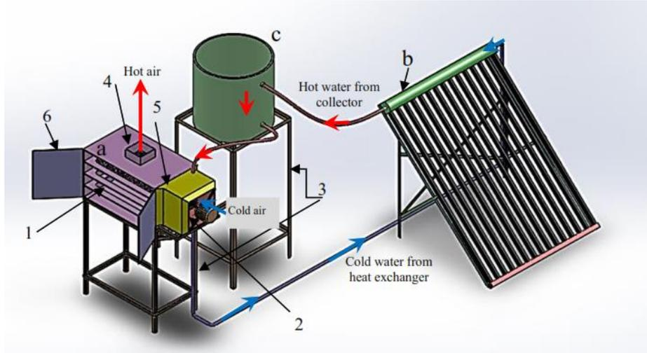
Figure 11. The schematic of solar cabinet dryer including a) Dryer: 1- sample trays and cabinet, 2- fan, 3- chassis, 4- exhaust channel, 5- Heat exchanger, 6- doors; b) ETSC; c) Storage tank and PCM container inside (Iranmanesh et al., 2020).
