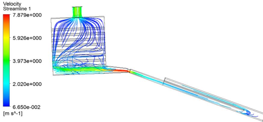
Figure 13. Velocity streamline of the chili drying chamber (Getahun et al., 2020)
