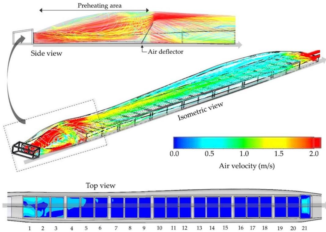
Figure 15. Visualization of airflow distribution and direction in the ISD (isometric and side view) and vertical flow through the 21 trays (top view) (Romuli et al., 2019).
