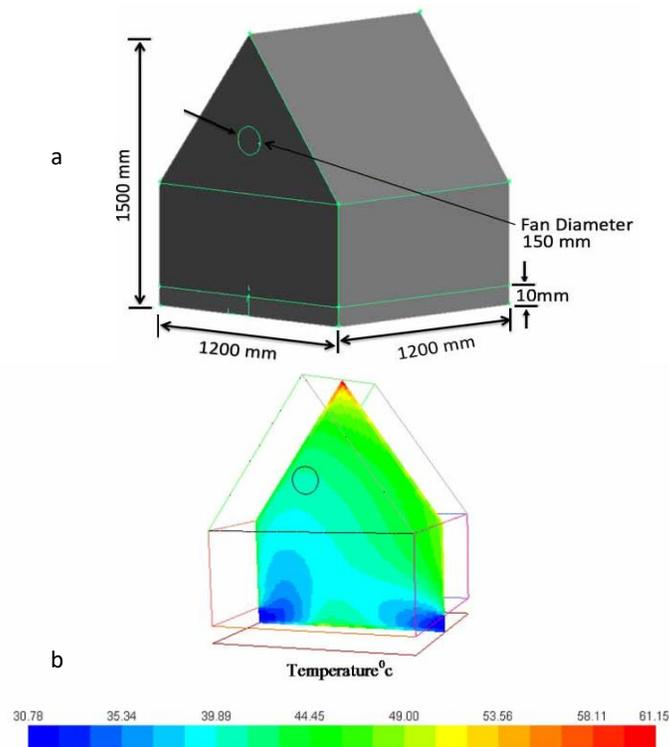
Figure 10:3-D model of the dryer (a) and temperature contour (b) of the midplane (Valarmathi, 2018).
