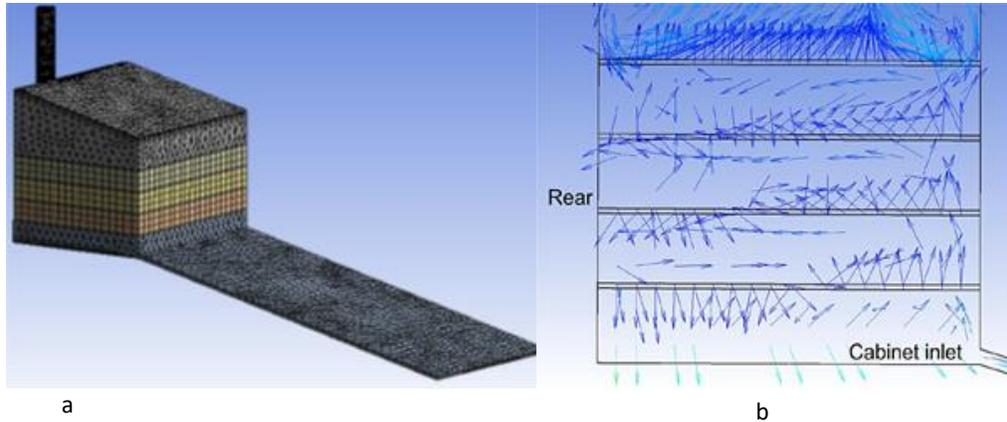
Figure 9: Geometry of a cabinet dryer (a) and air flow profile at the center plane (b) of a cabinet dryer (Sanghi et al., 2018).
