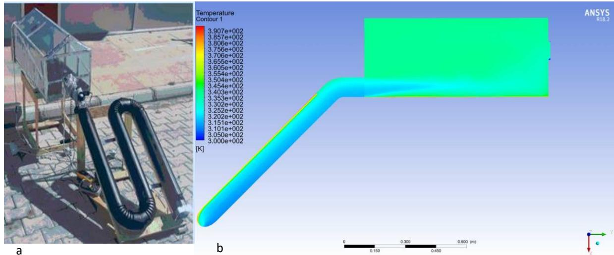
Figure 18: Apricot drying process in the solar greenhouse dryer, a) drying set up & b) drying temperature distribution inside the tube type collector (Khanlari et al., 2020).
