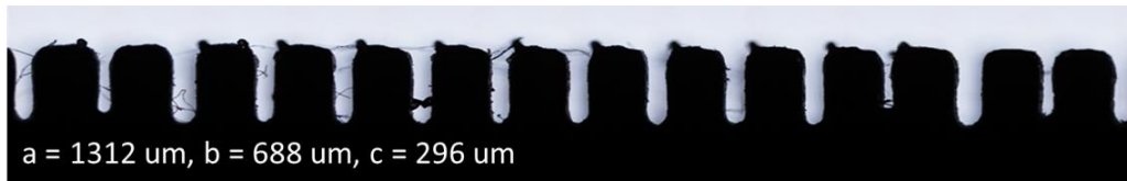
96 97 Fig. 1. Light microscopic image of the 3D printed, patterned casting knife *a = pattern height, b = pattern 98 width, c = pattern distance.
