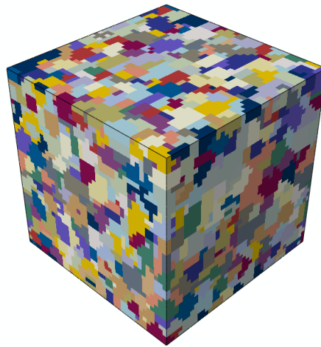
Figure 5: RVE showing the distribution of the grains in the synthetic microstructure. Grain distribution and their boundaries are depicted by the color overlay.
