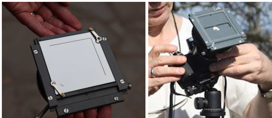
Figure 2.: Picture of a micro-interferometer plate in its mechanical support (left). This plate contains 49 different interferometric configurations that have been drilled by laser lithography. The plate and its support are mounted at the front of a classical digital camera (right picture).
