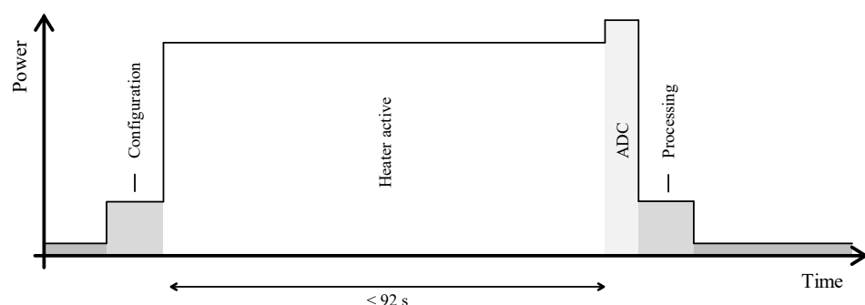
Figure 15. Power graph depicting the workings of a ‘forced’ gas measurement with a BME680 sensor [47]. A sensor remains in sleep and has no active operations until the controller commands, or forces, a measurement. A heated bed is required for an accurate gas value measurement. Heating the sensor element can take up to 92 s, consuming large amounts of energy.
