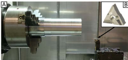
Figure 4: (a) Turning of C45 bars (DMG MORI NTX2000). (b) Geometry of tested inserts.
