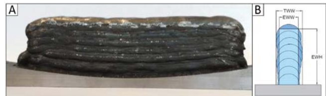
Figure 9: (a) Wall parts produced by WAAM. (b) Schematic representation of Effective Wall Width (EWW), Total Wall Width (TWW), and Effective Wall Height (EWH).
