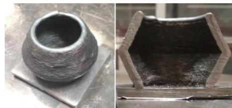
Figure 9 - Thin walled vase with inclined walls produced using conventional GMAW process
