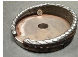
Figure 10 – Thick-walled flange produced using CMT process
