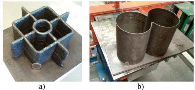
Figure 8 – Thin-walled part produced using a) conventional GMAW process; b) CMT process
