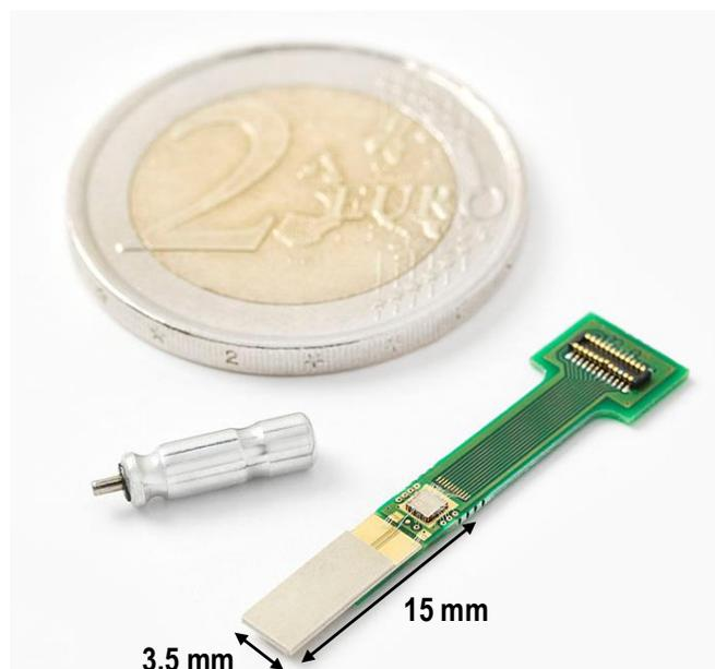
Fig. 4. An ultra-miniature wireless radio for ingestible applications [27].
