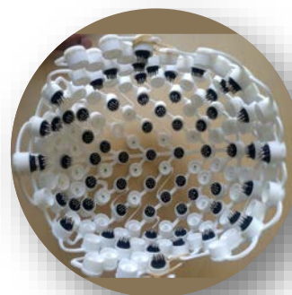
Figure 3: 128 dry electrode prototype wearable system developed by Datwyler
