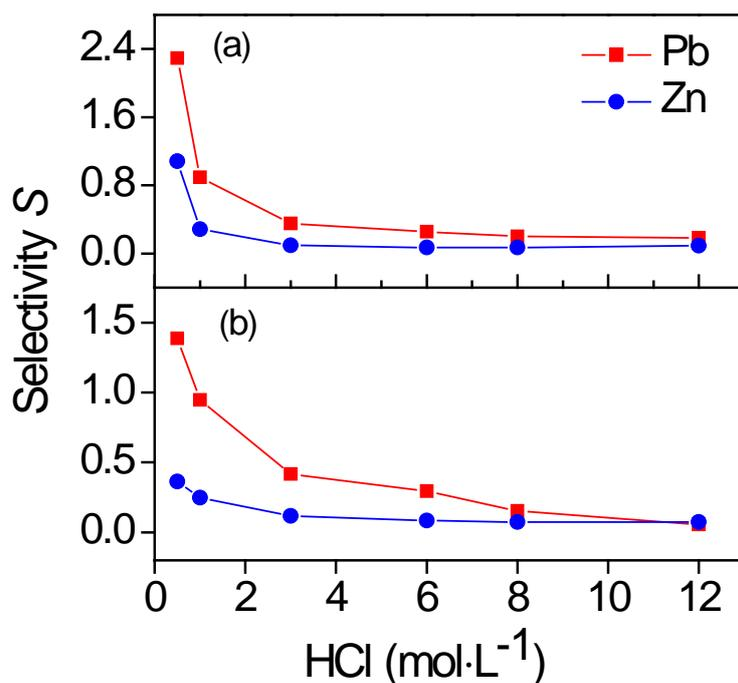
Figure 4: The selectivity  $S$  (Pb/Fe or Zn/Fe ratio) towards Pb (■) and Zn (●) over Fe, after leaching jarosite using (a) [A336][Cl] and (b) [C101][Cl] equilibrated with different HCl concentrations.
