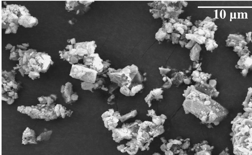
Figure 1: SEM micrograph of jarosite after drying (110 °C, 24 h) and milling (30 s, 1000 rpm).
