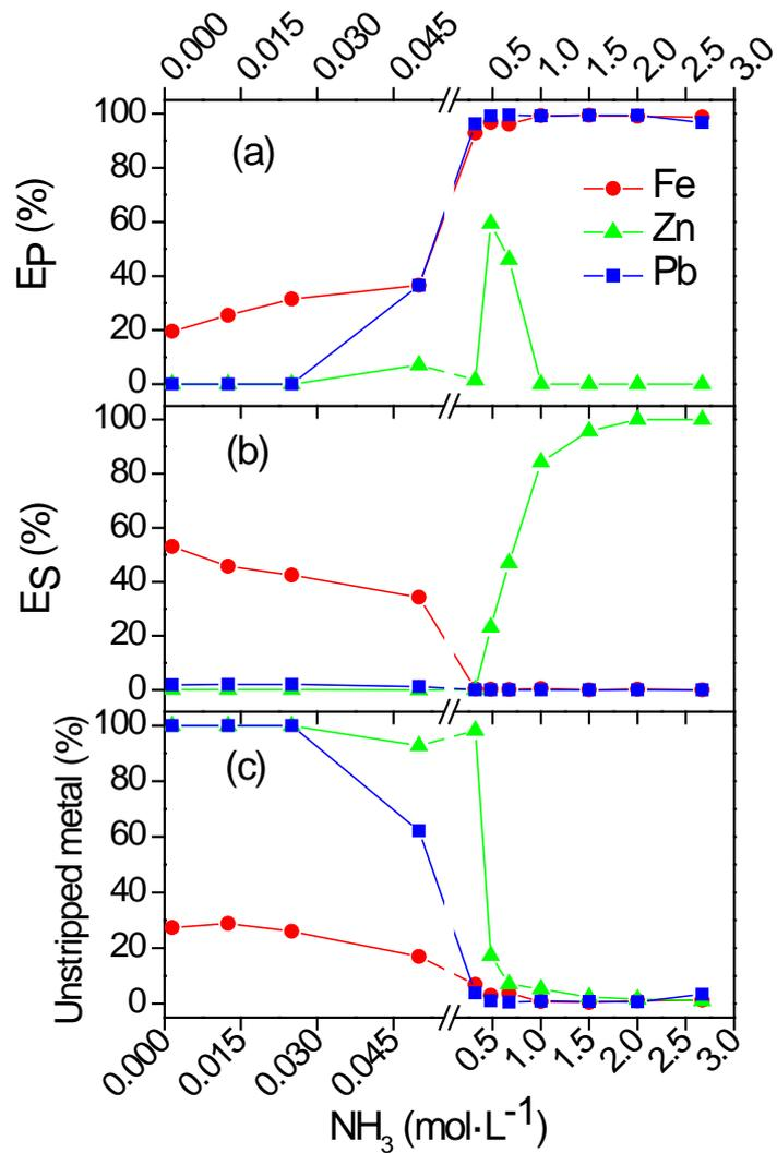
Figure 5: (a) The precipitating efficiency  $E_P$  (%), (b) the stripping efficiency  $E_S$  (%) and (c) the metals remaining in the stripped leachate (%) of Pb (■), Zn(▲) and Fe(●) from [C101][Cl] leachate to the aqueous phase when contacted with solutions with varying  $\text{NH}_3$  concentration. Stripping parameters: volume phase ratio  $\theta = 1$  (mL/mL), 1 h, 60 °C, 1500 rpm.
