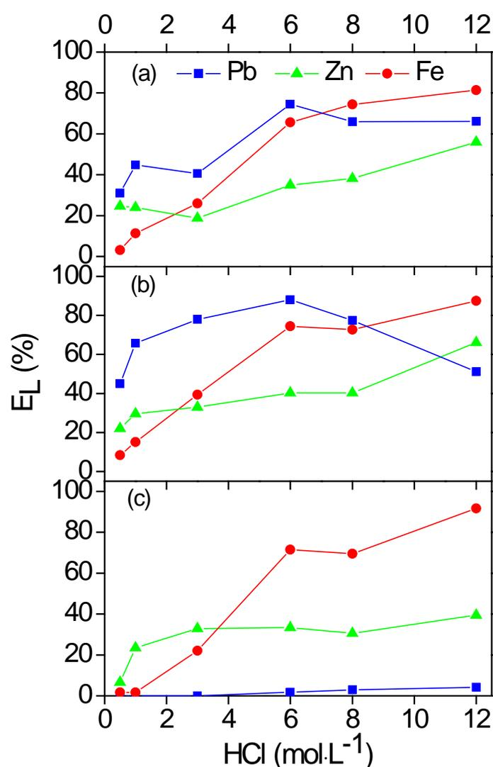
Figure 3: Leaching efficiency  $E_L$  (%) of Pb (■), Zn(▲) and Fe(●) from jarosite by (a) [A336][Cl], (b) [C101][Cl] and (c) TBP equilibrated with different HCl concentrations. Leaching parameters: L/S ratio  $10 \text{ mL g}^{-1}$ , leaching time 2 h,  $60^\circ\text{C}$ , 2000 rpm.
