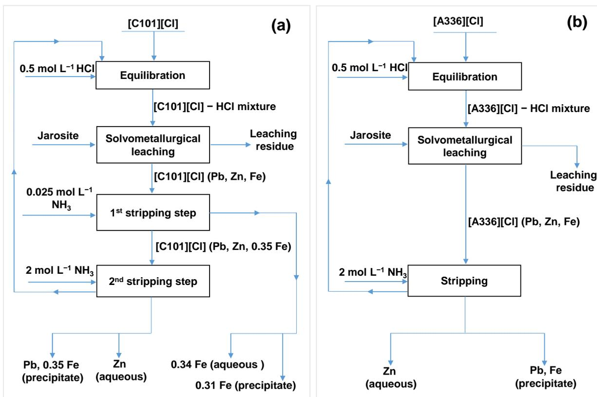
Figure 6: Flow chart for the recovery of lead, zinc and iron from jarosite by using (a) [C101][Cl] and (b) [A336][Cl] equilibrated with  $0.5 \text{ mol L}^{-1} \text{ HCl}$ .
