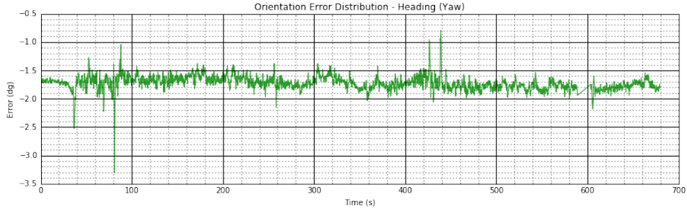
Figure 7: Orientation Error of the INS.
