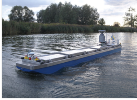
Figure 1: Scale Model Barge (Cogge).
