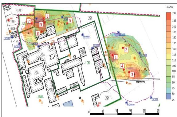
**Figure 1:** The site layout and electromagnetic readings
