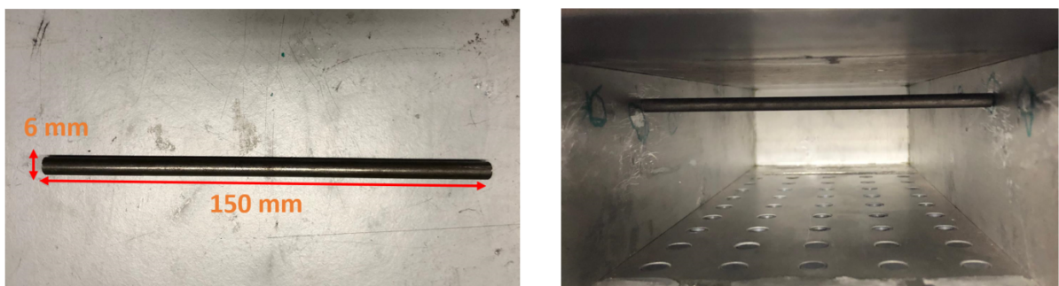
Figure 8: Realized bluff cylinder of D_c = 6 mm placed inside the duct section.
