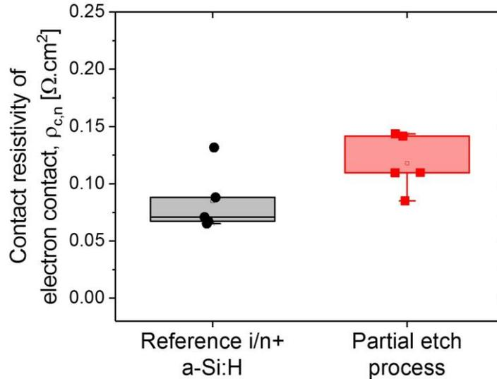
Figure 8. Plot of the contact resistivity values at the a-Si:H (*i/n*<sup>+</sup>) contact, comparing the partial etch process with reference.
