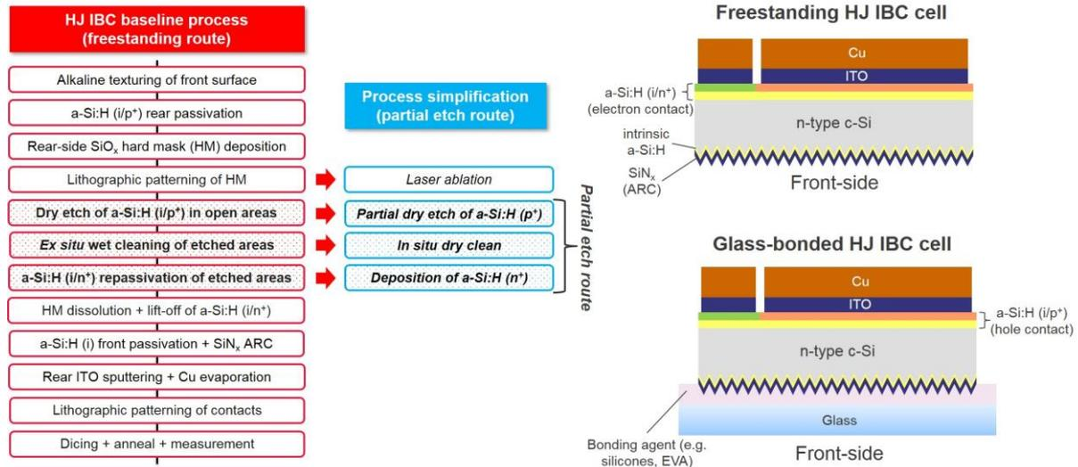
Figure 1. The baseline HJ IBC process flow (left). Process simplifications leading to an all-dry, litho-free, cost-effective process flow are also indicated (middle). Cross-sectional schematics of a freestanding and a glass-bonded HJ IBC cell are given on the right.
