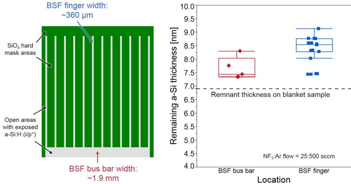
Figure 5. Schematic on the left shows design of the rear-side of our small-area IBC rear-side a-Si finger pattern. Plot on right shows the remaining a-Si:H thickness after the partial etch process at the BSF finger and bus bar. The dashed line indicates the expected thickness.
