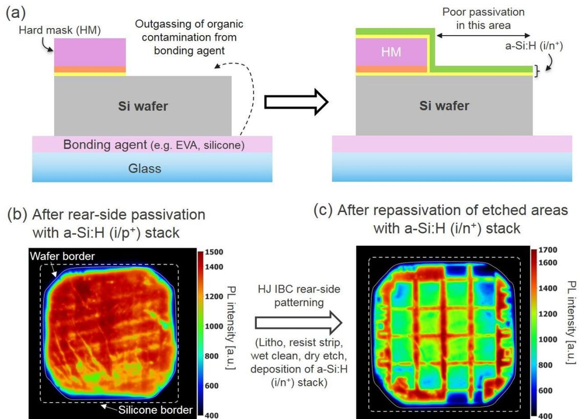
Figure 3. (a) Schematics depicting outgassing of organic contamination from the bonding agent onto the re-exposed c-Si surfaces and the resulting poor re-passivation. (b) and (c) PL images showing the passivation quality during rear-side processing of HJ IBC cells on glass-bonded silicon.
