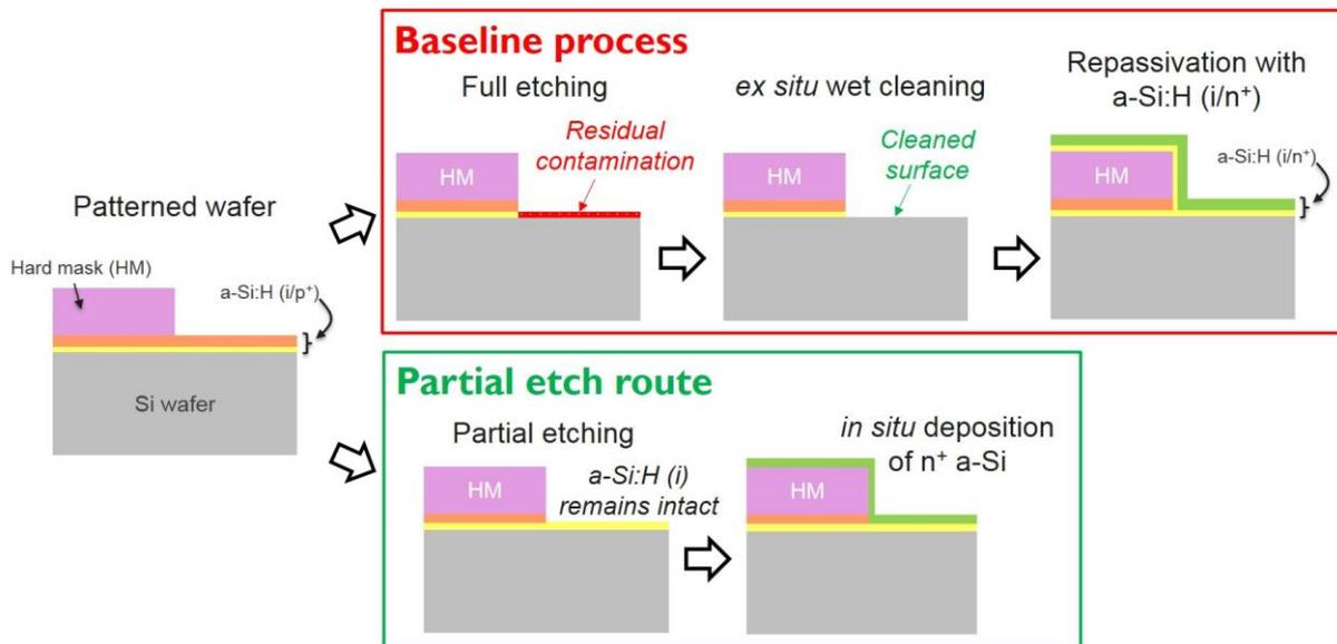
Figure 2. Schematics depicting the steps after HM patterning till the realization of interdigitated strips of a-Si:H (i/p<sup>+</sup>) and a-Si:H (i/n<sup>+</sup>), comparing the conventional baseline route with the proposed partial etch route.
