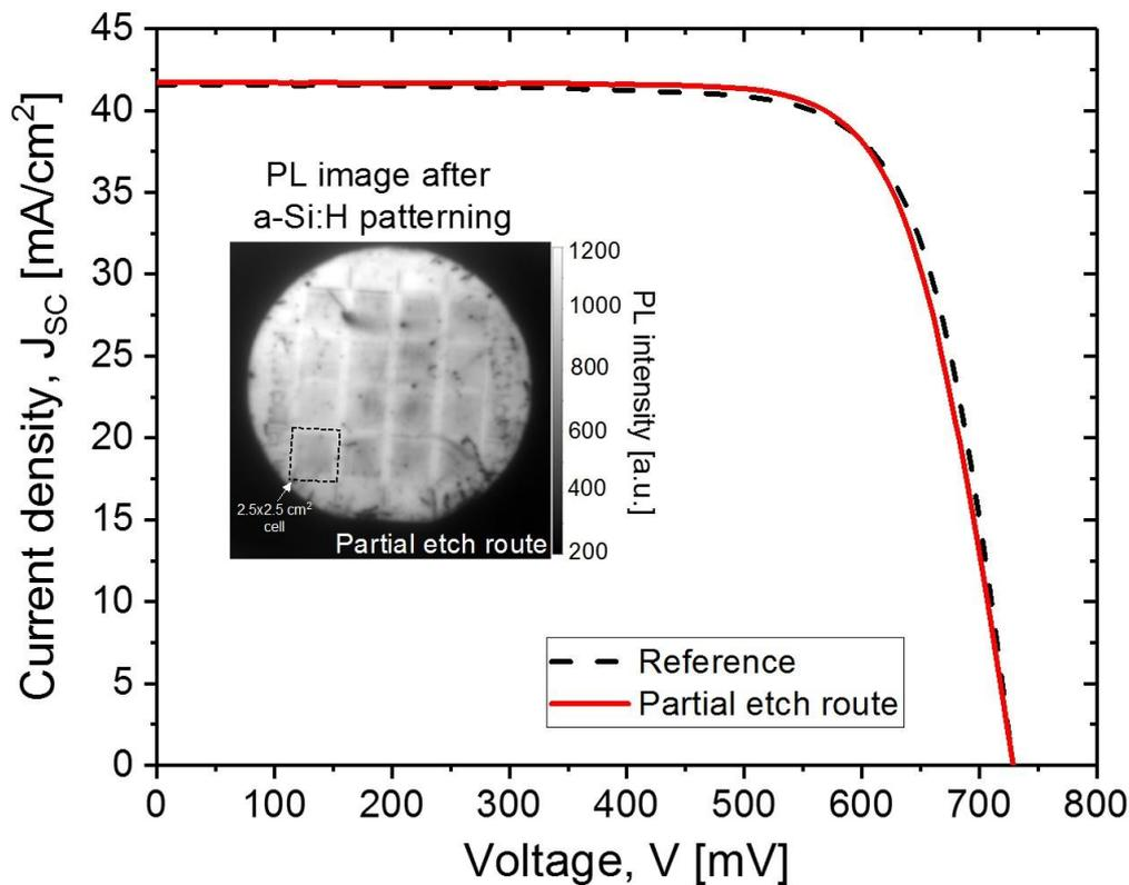
Figure 9. The current-voltage characteristics under AM1.5G illumination of the best cell from the partial etch route and that from the reference conventional process sequence. Inset shows the uncalibrated PL image of a wafer after the rear-side a-Si:H patterning, from the partial etch route.
