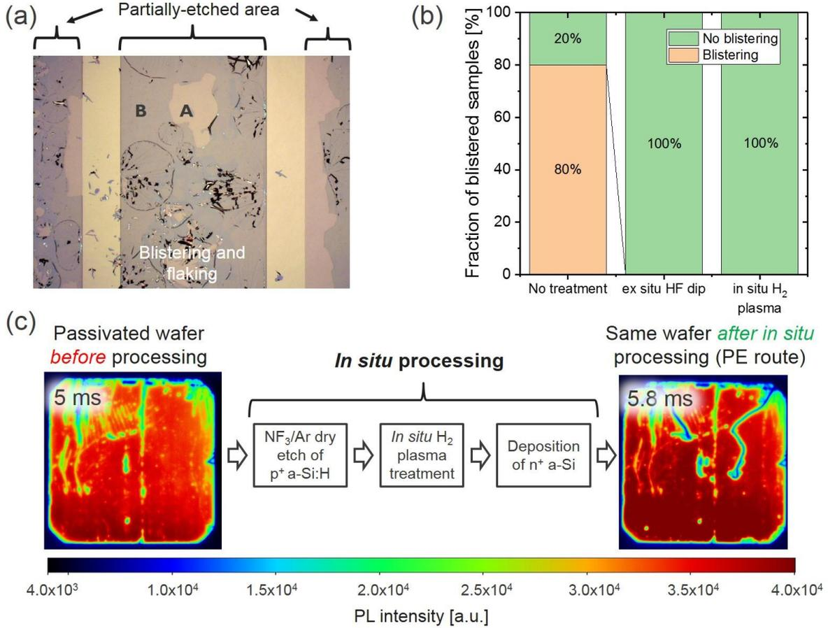
Figure 7. (a) Optical microscopy image showing the blistering of *p*-doped a-Si:H deposited on remnant a-Si:H after the partial etch of *n*-doped a-Si:H, when immersed in HF solution at the end of the process. (b) Plot of the fraction of blistering incidents as a function of surface treatment after partial etching. (c) PL images before and after the fully *in situ* partial etch process sequence, including the short H<sub>2</sub> plasma dry clean.
