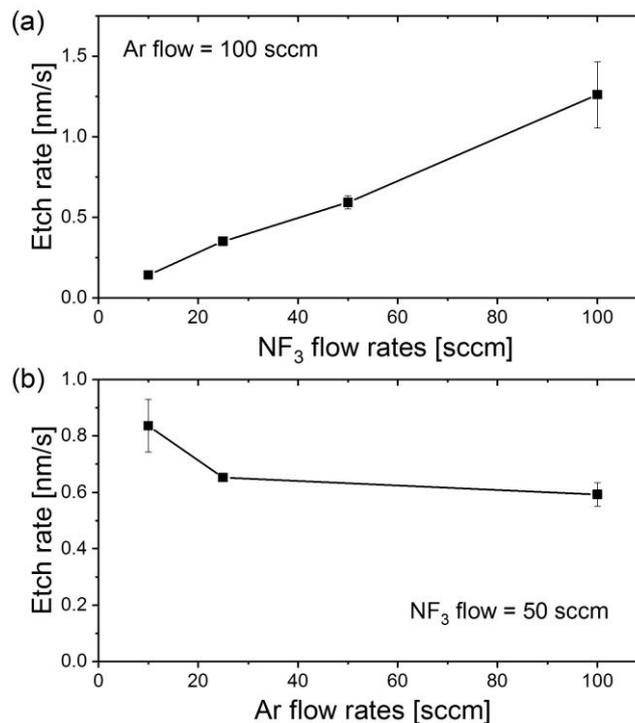
Figure 4. Etch rates of a-Si:H ( $n^+$ ) when dry etching with  $\text{NF}_3/\text{Ar}$  plasma with (a) different  $\text{NF}_3$  flow rates (at a constant Ar flow rate of 100 sccm) and (b) different Ar flow rates (at a constant  $\text{NF}_3$  flow rate of 50 sccm).
