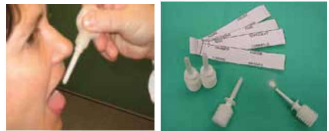
Figure 9. A retronasal test device based on food powders. The powders are applied by means of squeezable vials onto the subject's tongue.
