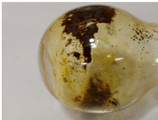
Figure S10. Magnet powder obtained after refluxing an epoxy-bonded magnet in an aqueous NaOH solution. The powder shows clear signs of oxidation.
