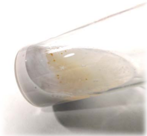
Figure S11. White precipitate of metal sulfates after dissolving PA12 from a PA12-bonded magnet by concentrated sulfuric acid.
