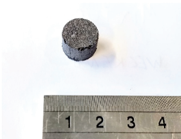
Fig. 4 One of the produced compression-bonded NdFeB magnets from recycled magnet powder.
