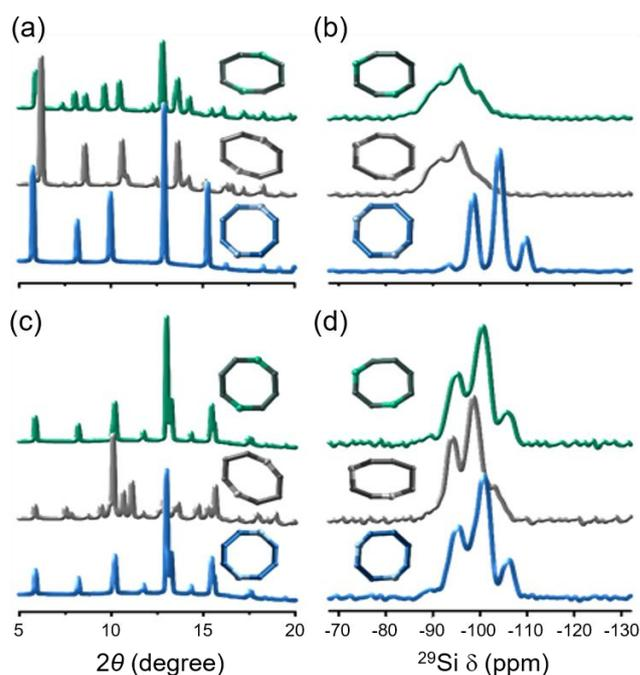
**Fig. 2** PXRD patterns (left) and <sup>29</sup>Si MAS NMR spectra (right) of (a) and (b) Na-GIS-3.0 and (c) and (d) Rb-GIS-3.0 in hydrated (blue), dehydrated (gray), and CO<sub>2</sub>-loaded (green) states. Also shown are the 8-MR windows of the GIS framework as seen in crystallographic a and b directions with Al positions highlighted.
