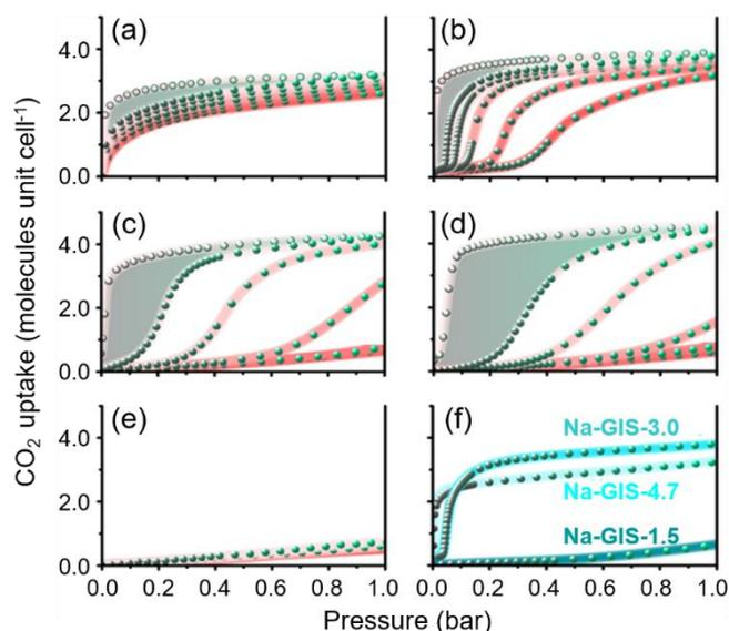
**Fig. 1** Adsorption isotherms on (a) Li-, (b) Na-, (c) K-, (d) Rb-, and (e) Cs-GIS-3.0 as a function of CO<sub>2</sub> molecules per unit cell. Adsorption, filled symbols; desorption, open symbols. Red traces indicate measurement temperatures, from light to dark corresponding to 25, 35, 50, 60, and 75 °C. Green shaded areas show hysteresis between ad- and desorption at 25 °C. (F) Comparison of adsorption isotherms of Na-GIS-1.5 (dark), Na-GIS-3.0 (medium), and Na-GIS-4.7 (light).
