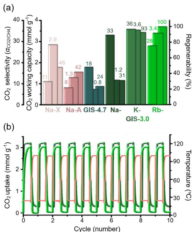
**Fig. 4** (a) CO<sub>2</sub> Selectivity ( $\alpha$ ), CO<sub>2</sub> working capacity, and regenerability in columns (from left to right) of Na-X, Na-A, Na-GIS-4.7, Na-GIS-3.0, K-GIS-3.0, and Rb-GIS-3.0. (b) CO<sub>2</sub> adsorption-desorption cycles for K-GIS-3.0 (dark green) and Rb-GIS-3.0 (light green) with adsorption at 25 °C using a 50:50 CO<sub>2</sub>/CH<sub>4</sub> mixture and desorption at 100 °C using pure CO<sub>2</sub>.
