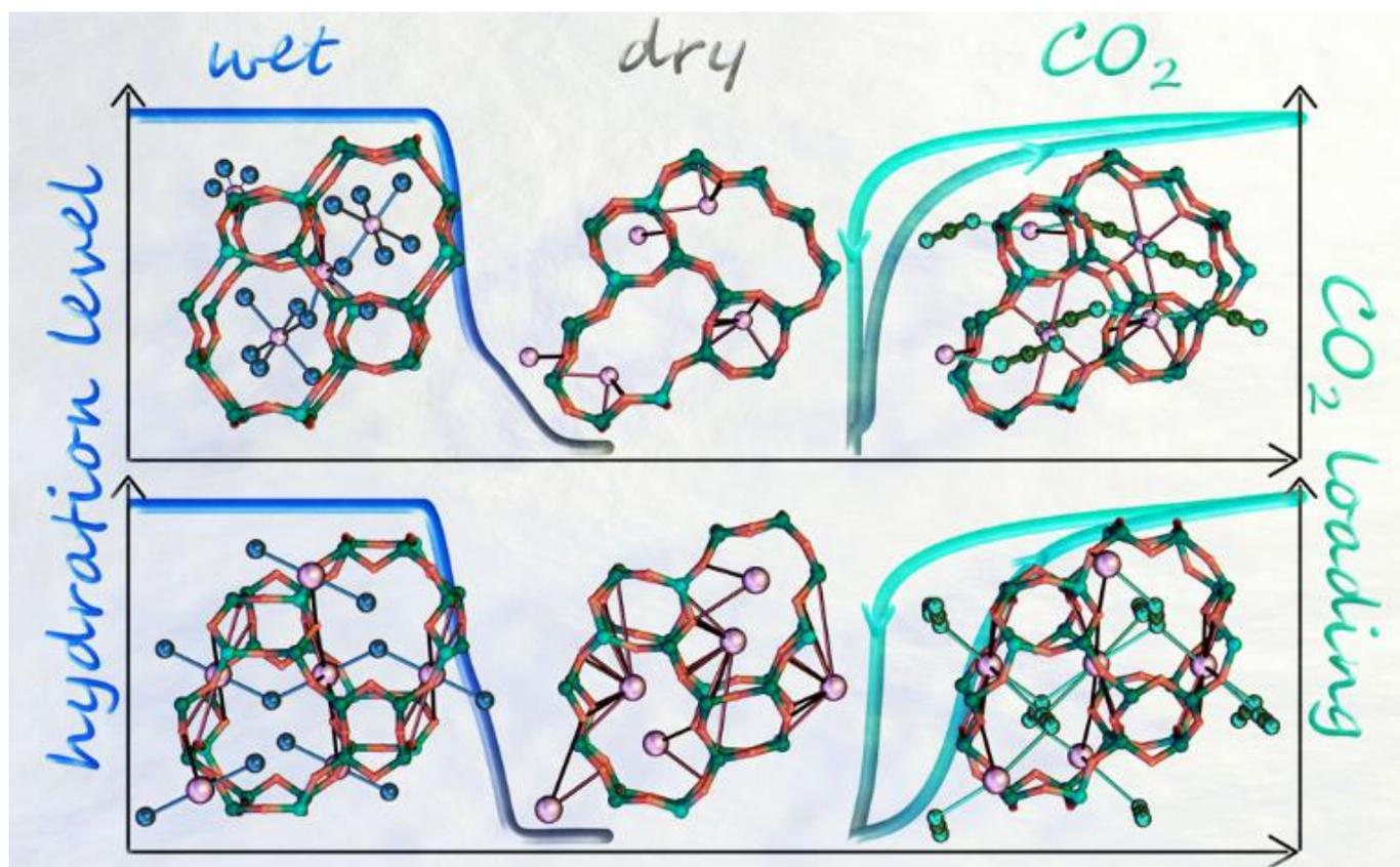
**Fig. 3** The structures of Na-GIS-3.0 (top) and Rb-GIS-3.0 (bottom) in hydrated (left), dehydrated (middle) and CO<sub>2</sub>-loaded (right) states. The blue and green traces represent thermogravimetric dehydration and CO<sub>2</sub> adsorption–desorption isotherms, respectively.
