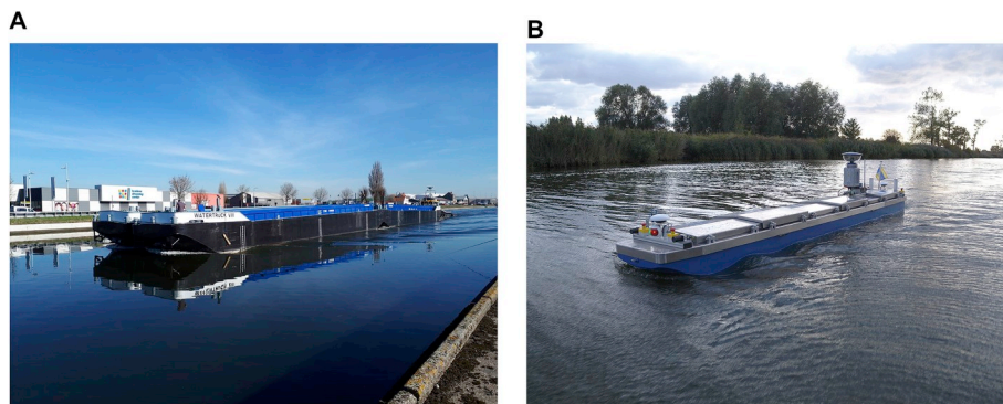
Fig. 2. (a) Watertruck+ convoy: consisting of four CEMT I barges pushed by one push boat (slightly visible on the right hand side), and (b) the KU Leuven scale model.
