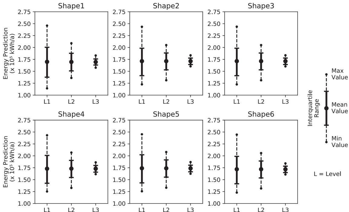
Fig. 7. Effect of the uncertainty in design parameters on the performance prediction.
