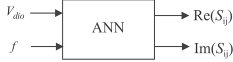
FIGURE 10 Neural model for bias dependent modeling of a Si fin field-effect transistor varactor: artificial neural network (ANN) used for simultaneously modeling the real and imaginary parts of each S -parameter
