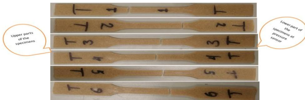
Figures 12: Tensile test specimens after testing
