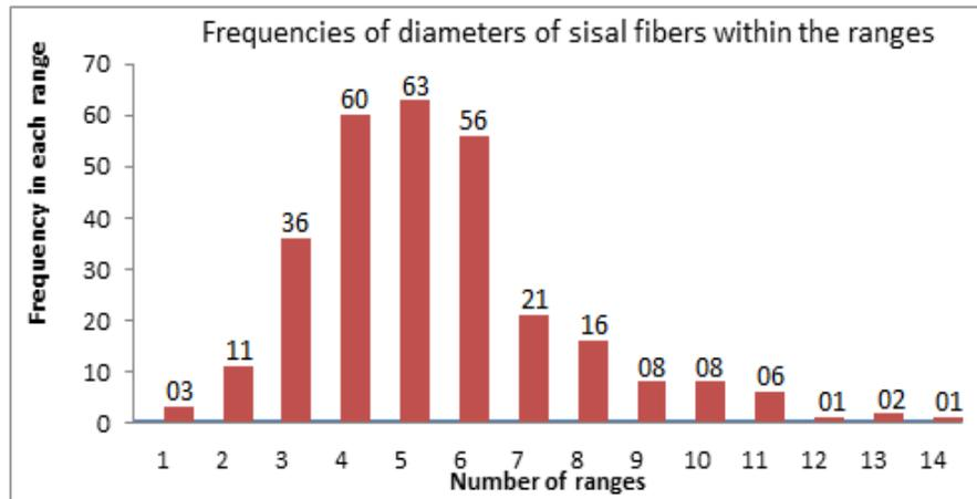
Figure 6: Frequencies of diameters of sisal fiber
