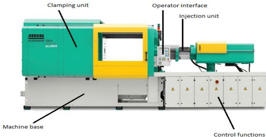
Figure 8: The Injection Molding Machine
