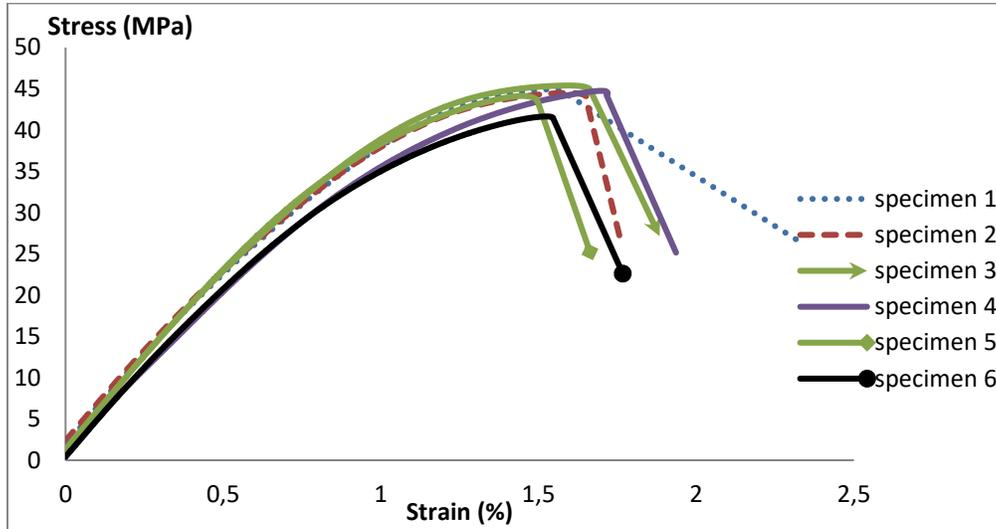
Figure 11: Stress-strain graphs of tensile specimens
