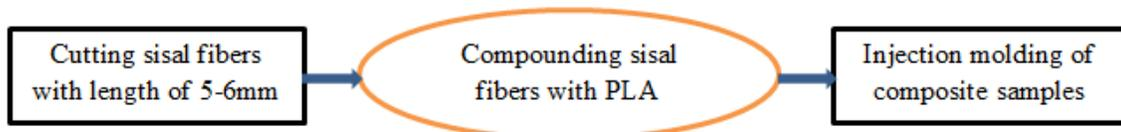
Figure 7: Major steps involved in fabrication of bio-composite samples
