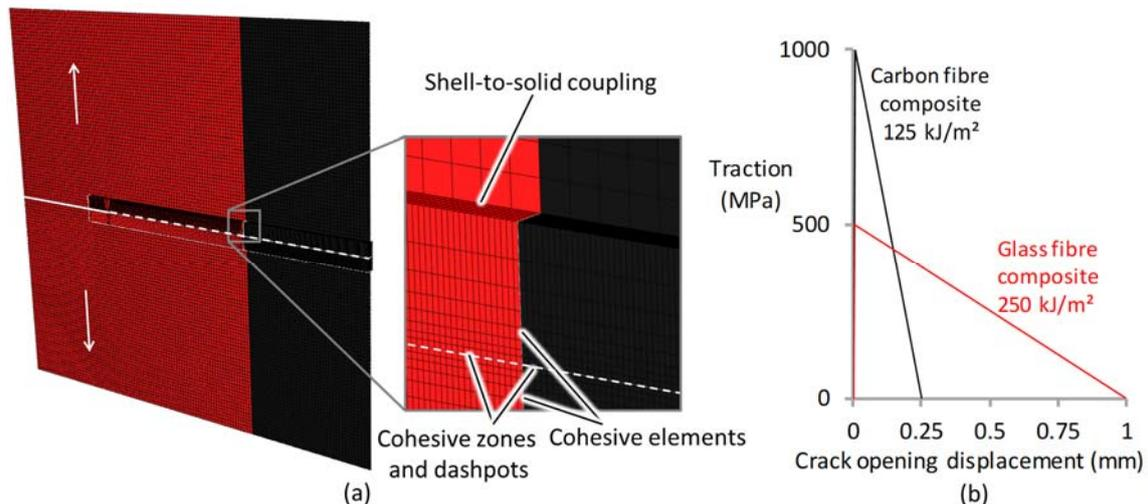
**Figure 1: The finite element model for translaminar fracture: (a) 3D view with the arrows indicating the loading points and (b) the cohesive laws used for the carbon and glass fibre composites. The full white line indicates the initial crack and the dashed white line the fracturing region. The dashpots are not shown.**
