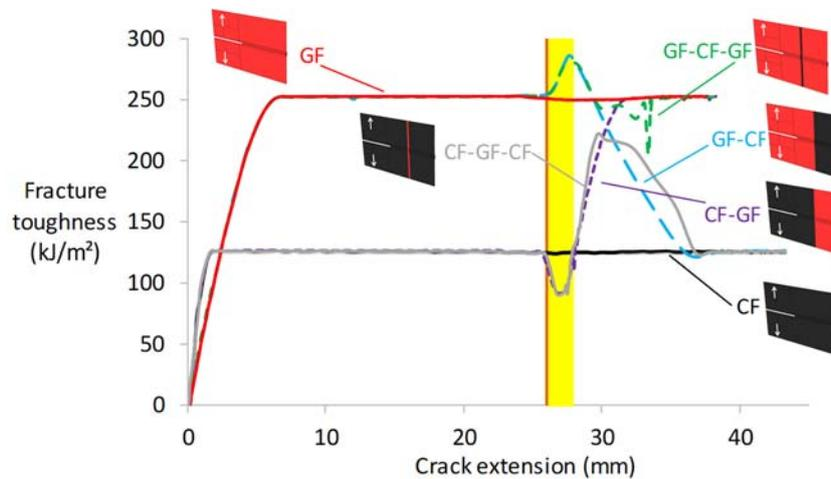
**Figure 4: Fracture toughness evolution of the six different finite element models as a function of crack extension. The vertical orange line indicates the start of the material transition in the GF-CF and CF-GF models, whereas the yellow region indicates the width of the strips in GF-CF-GF and CF-GF-CF models.**
