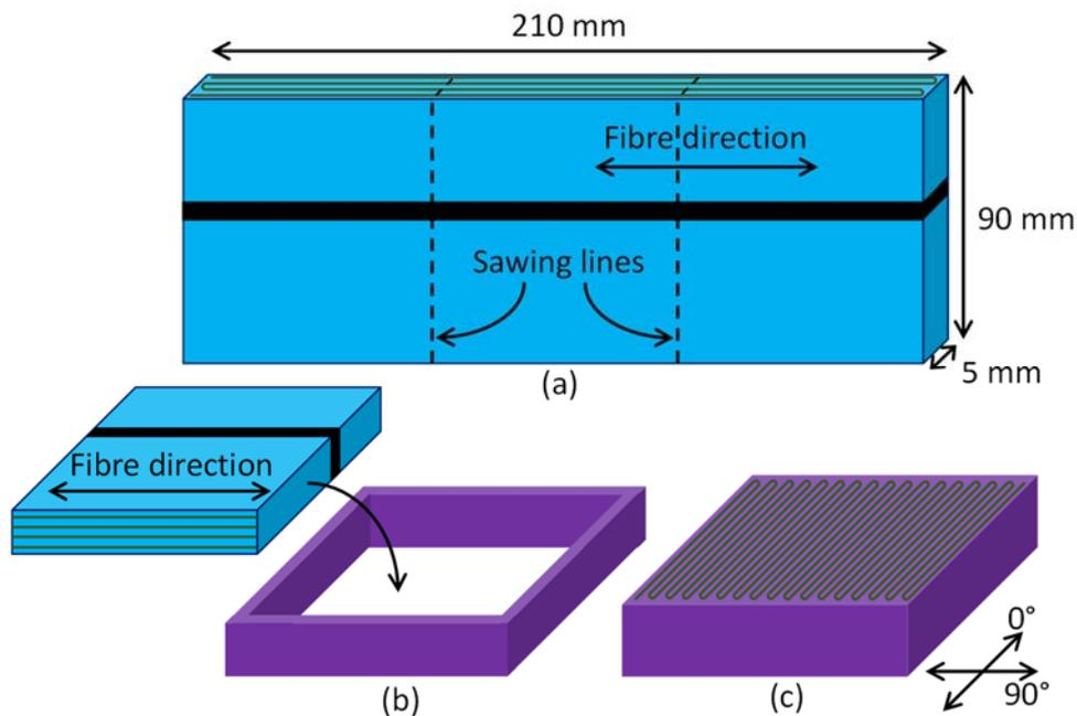
**Figure 6: Schematic overview of the first two printing steps: (a) printing of the middle  $0^\circ$  block, (b) printing the first half of one  $90^\circ$  block to insert a  $0^\circ$  block, and (c) printing the second half of one  $90^\circ$  block by overprinting of the  $0^\circ$  block.**
