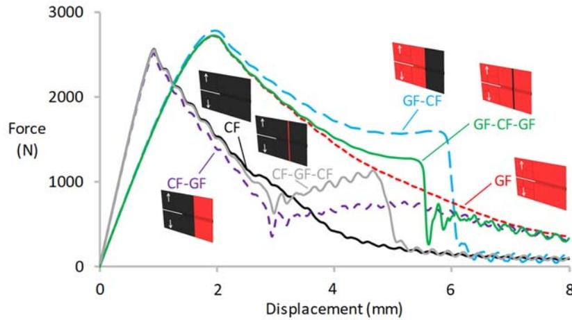
**Figure 3: Force-displacement diagrams of six different finite element models.**
