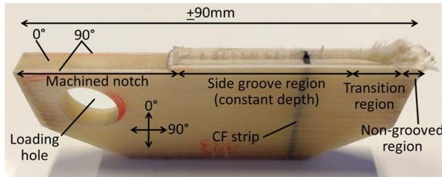
**Figure 7:** Half of a fractured compact tension specimen, showing the layup, the location of the strip, the machined notch and the side groove. The scale bar is only approximate due to the 3D nature of the photograph.
