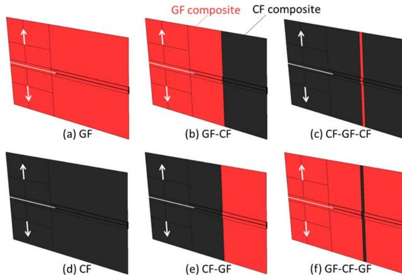
**Figure 2: Six finite element models with no or with different material transitions: (a) GF, (b) GF-CF, (c) CF-GF-CF, (d) CF, (e) CF-GF, and (f) GF-CF-GF. The initial crack is indicated with a white line, with the crack growing from the left- to the right-hand side.**
