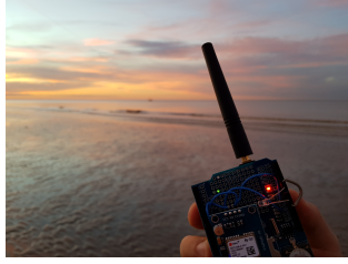
(a) Receive side implemented on a hand-held device to carry out the measurement campaigns.
