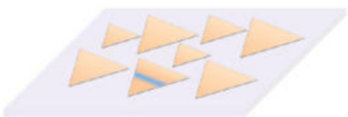
Figure 2-9: Selective growth in focused ion beam (FIB) pre-patterned 2D islands. Reproduced from doi: 10.1021/acsnano.6b06496.
