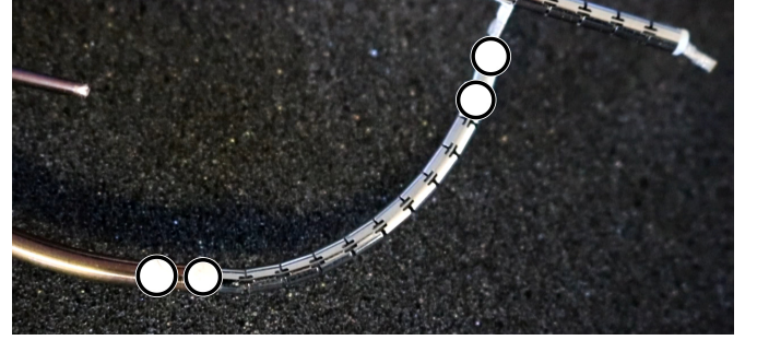
Fig. 7: Markers for image tracking on end-effector
