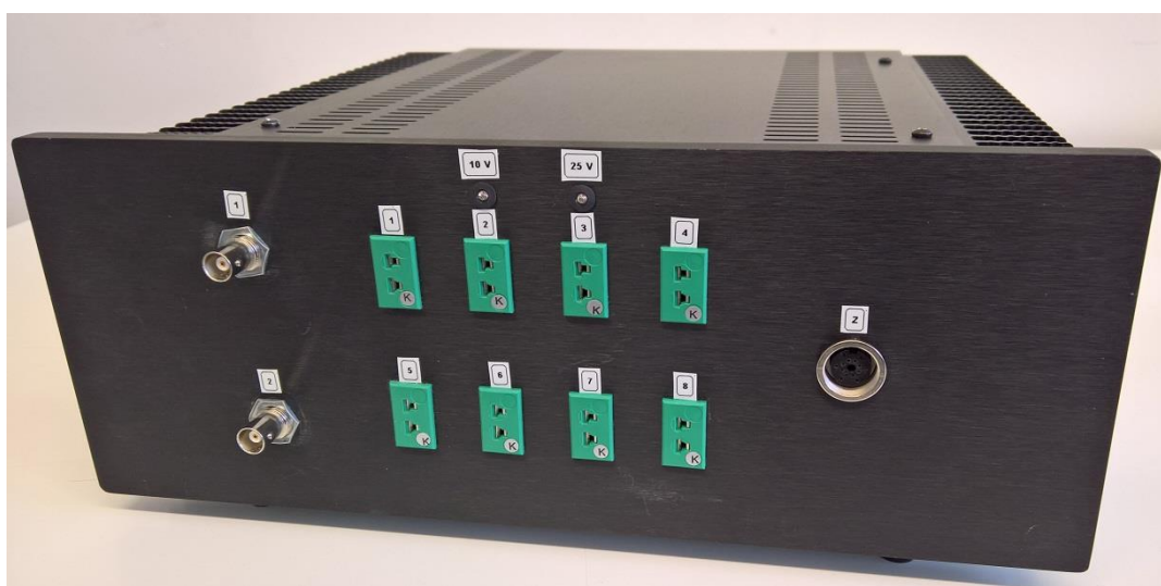
Figure 2-5 Picture of the assembled electronic base unit (EBU).
