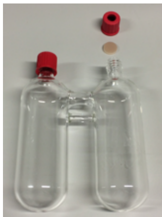
Figure 7.4 Large two-chamber reactor [43-44] with an inner volume of approximately 400 mL
