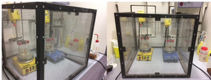
Figure 7.1. Performing a gas-mediated reaction in a two-chamber reactor behind a blast screen.
