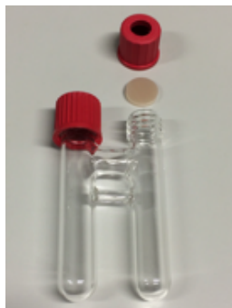
Figure 7.2. Two-chamber reactor [43-44] with an inner volume of approximately 20 mL
