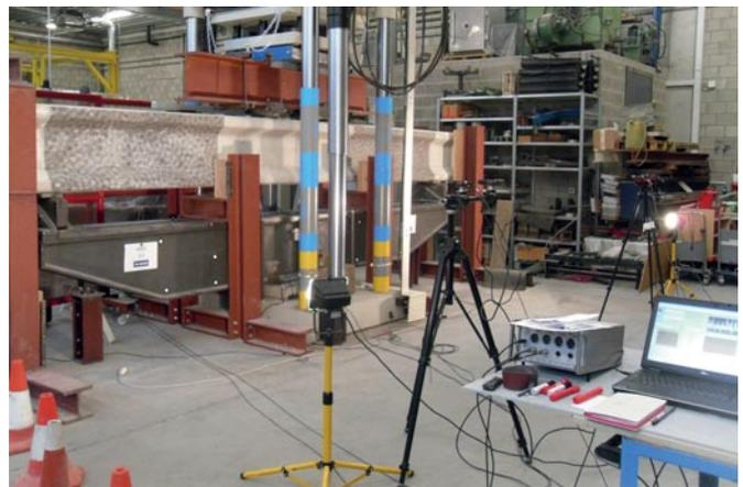
(b) Camera setup for DIC measurements
