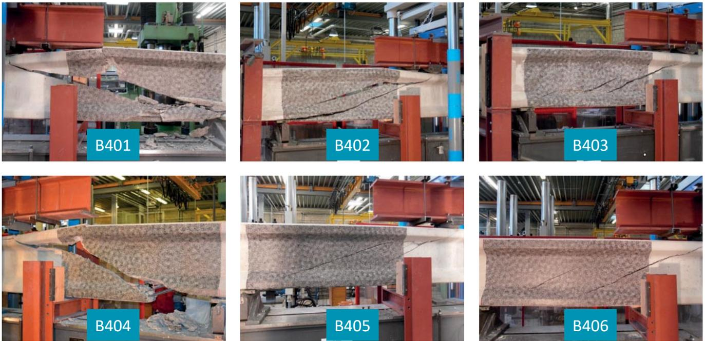
Fig. 9: Experimentally observed shear failure mode of the tested beams.
