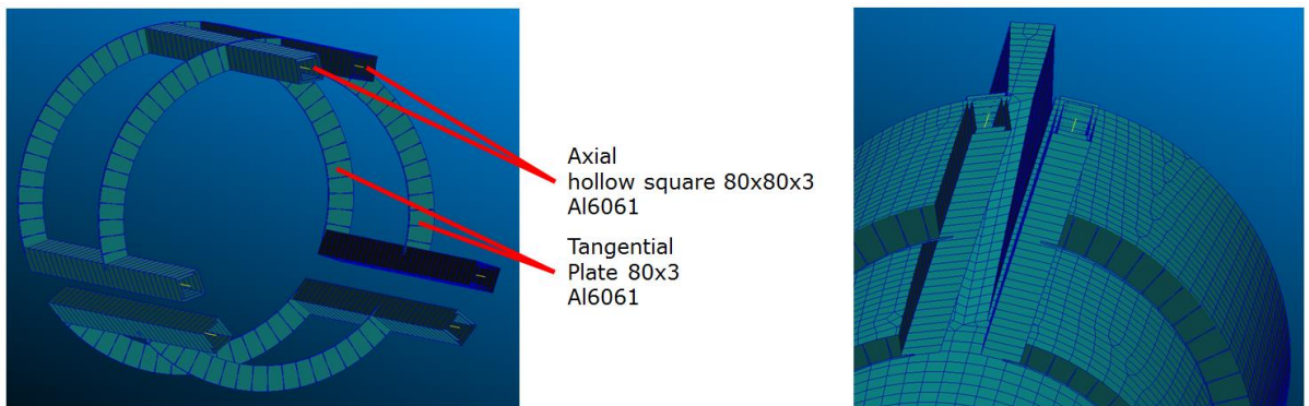
Fig 11. Stiffeners as built in the FEM.
