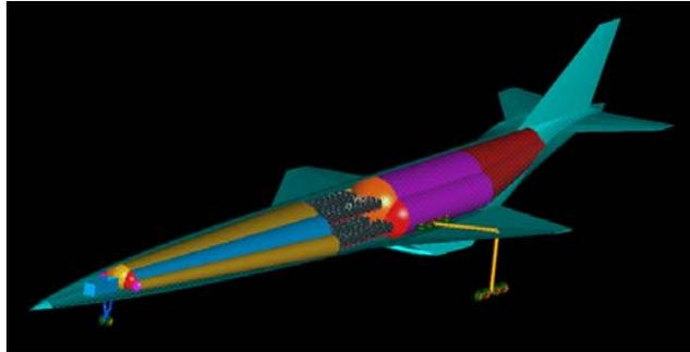
**Fig. 5:** A Multi-lobe Tank extension module is successfully used for fast design of the internal volume (DLR-SART).
