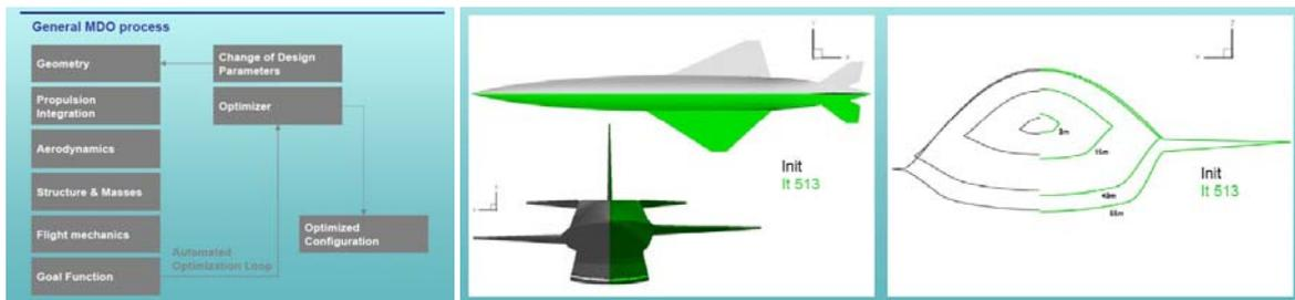
**Fig. 1:** MDO process for the airframe and first results using a single point multidisciplinary optimization. (DLR-AS)
