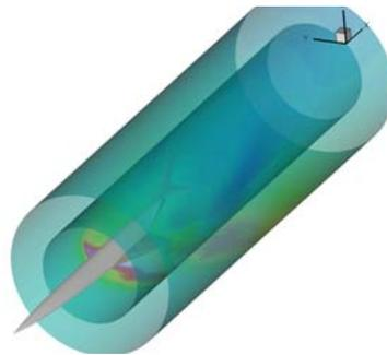
**Fig. 6:** CFD near field pressure footprint extraction from a DLR CFD solution (ONERA).
