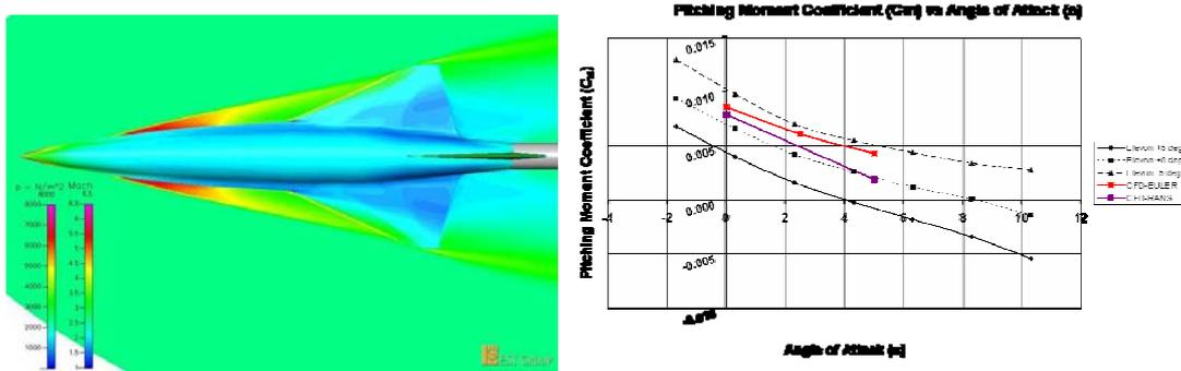
Fig. 9: Surface pressure distribution, left picture, and pitching moment coefficient vs. AoA.(ESA-ESTEC)
