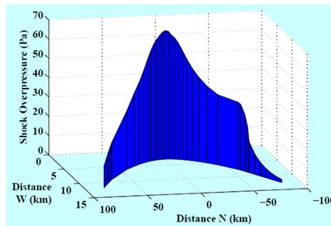
**Fig. 7:** example of delta pressure carpet prediction (UPMC).
