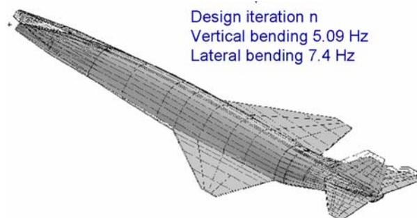
**Fig. 4:** Preliminary bending analysis of the aircraft' structure (FOI).
