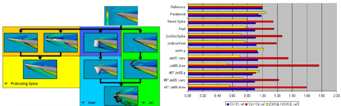
**Fig. 8:** Pedigree of spike design. Left: geometries, right: impact on aircraft performances. (DLR-AS)
