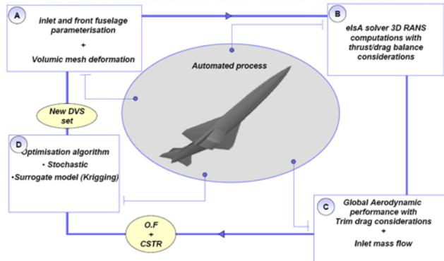
**Fig. 3:** MDO process for the propulsion integration. (ONERA)
