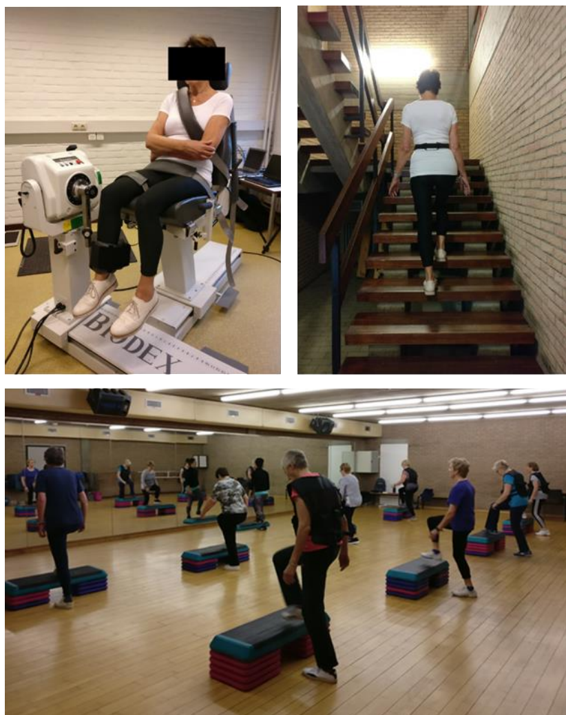
Figure 1: Setup of the isokinetic dynamometer (top left). The timed stair ascent task with lower back-mounted accelerometer (top right). Impression of a training session in week 10 (bottom).
