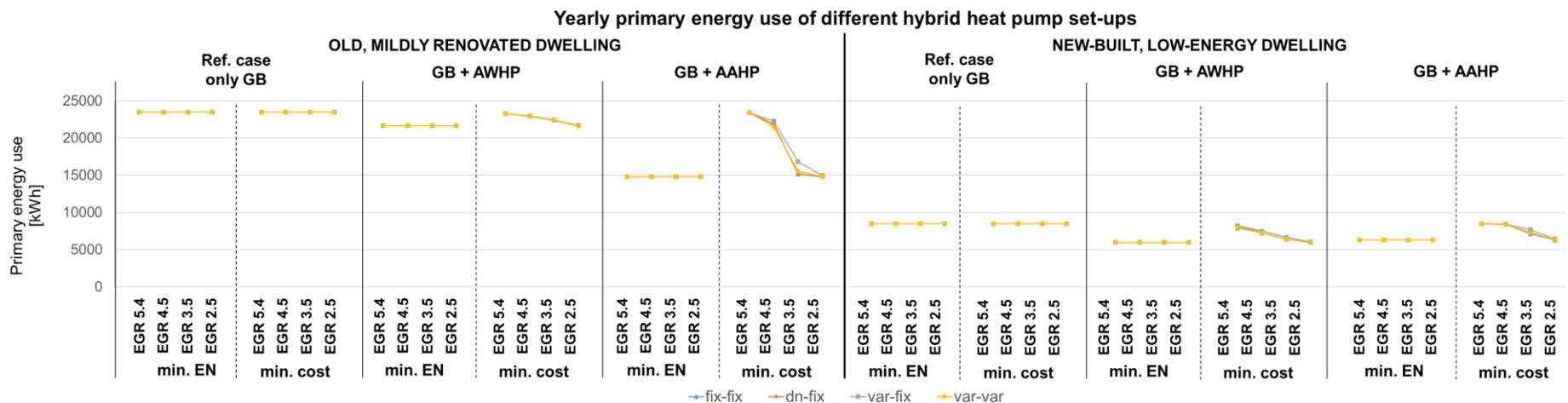
Figure 8 Yearly primary energy use of AWHP or AAHP in a hybrid heating system, according to different objectives and different price scenarios, in an old, mildly renovated dwelling, or in a new-built, low-energy dwelling. The reference heating system that only uses a gas boiler serves as a benchmark.
