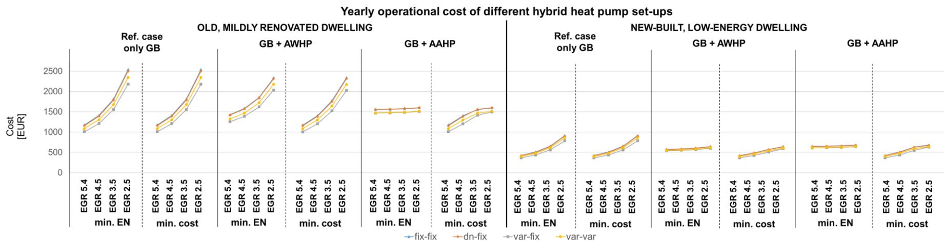
Figure 9 Yearly operational cost of AWHP or AAHP in a hybrid heating system, according to different objectives and different price scenarios, in an old, mildly renovated dwelling, or in a new-built, low-energy dwelling. The reference heating system that only uses a gas boiler serves as a benchmark.
