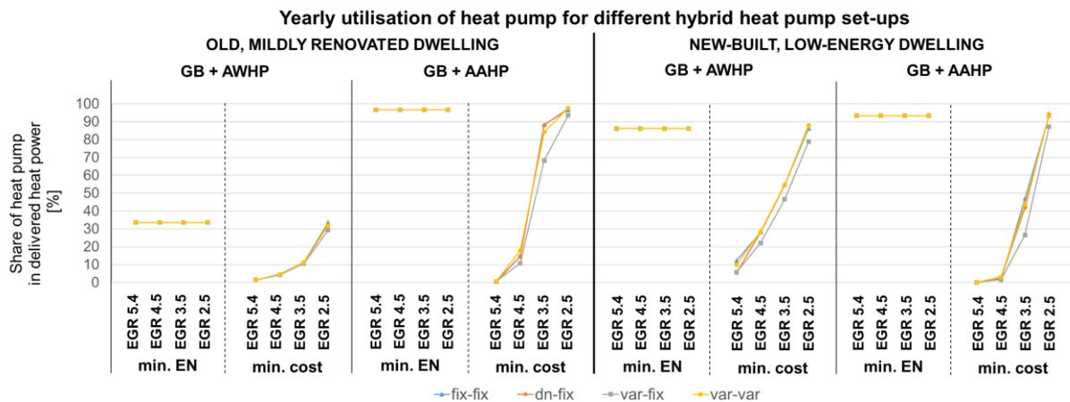
Figure 6 Yearly utilisation of AWHP or AAHP in a hybrid heating system, according to different objectives and different price scenarios, in an old, mildly renovated dwelling, or in a new-built, low-energy dwelling.
