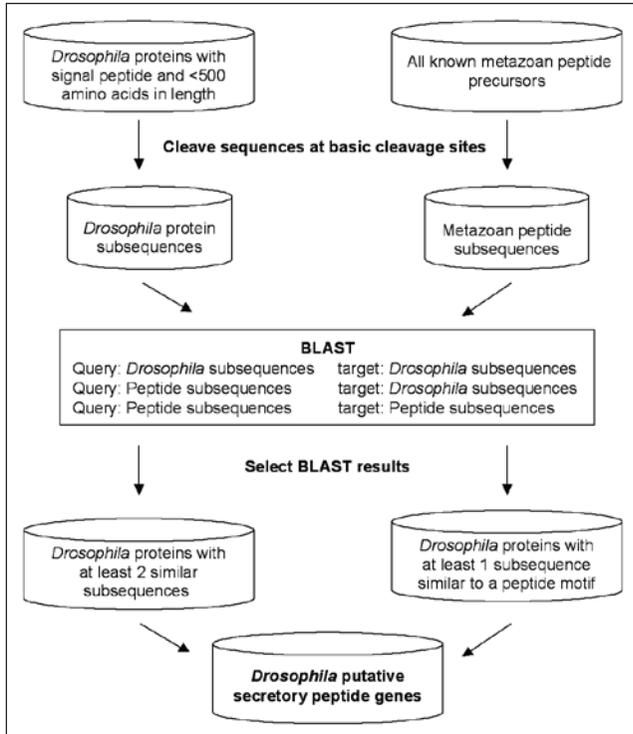
Figure 1. Schematic representation of the in silico neuropeptide searching program developed by Liu et al.<sup>5</sup>
