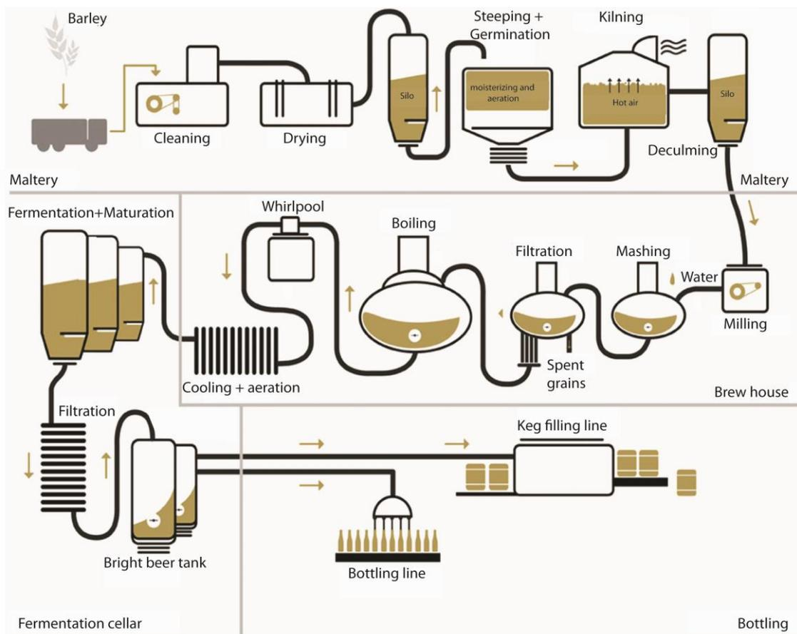
**Figure 1: Schematic overview brewing process.** Within the maltery, raw grains are malted before being transferred towards the brewery. Within the brew house, malt and other grains are first milled and mixed with warm water in the mashing-in vessel. Next, wort is filtered and boiled after which it is cooled, aerated and transferred to a fermentation tank. After fermentation and maturation, beer is filtered and bottled or transferred to kegs for consumption (adjusted from (123)).
