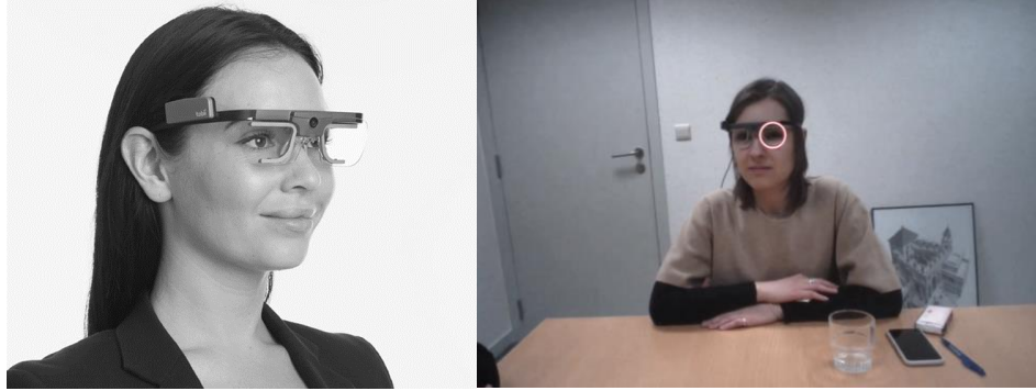
Figure 2.2: An example of eye-tracking glasses ( Tobii Pro Glasses 2 ) (left picture) and the eye-tracking recording (right picture). Participant's gaze fixation is indicated with a colored dot (also called gaze cursor ).
