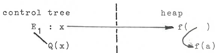
Fig. 6.c. A garbage collector can recuperate parts of the heap and can simplify the access to the structures.
