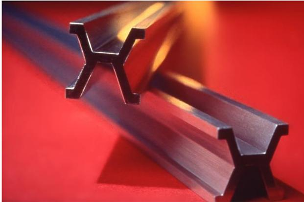
Figure 1.8. The International Prototype Platinum-Iridium meter bar. Image courtesy of NIST.
