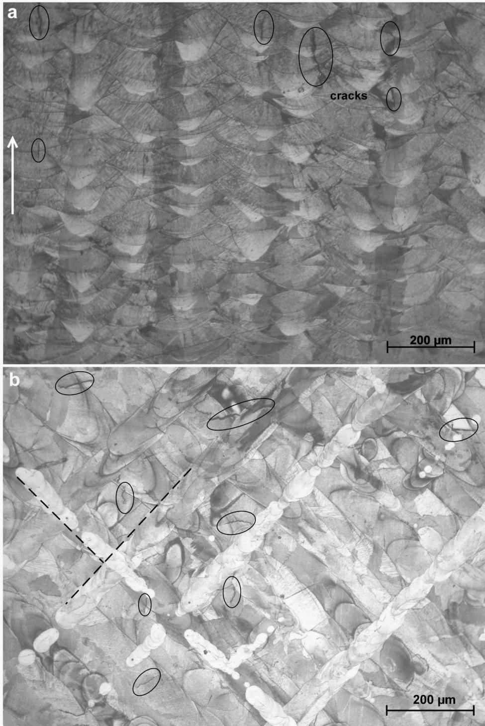
**Fig. 5.** OM images showing the microstructure of (a) vertical and (b) horizontal sections fabricated at a scanning speed of 200 mm/s and hatch spacing of 90 μm; the white arrow indicates the building direction.
