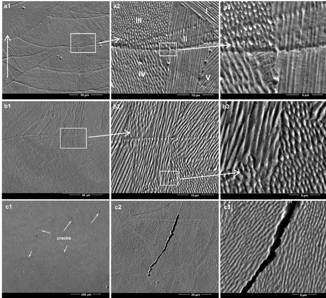
**Fig. 6.** SEM images showing the microstructures of vertical and horizontal sections fabricated under the optimum parameters: (a1–a3) vertical section (regions I–V presented different types of solidification microstructures); (b1–b3) horizontal section; (c1–c3) microcracks observed on the horizontal section.
