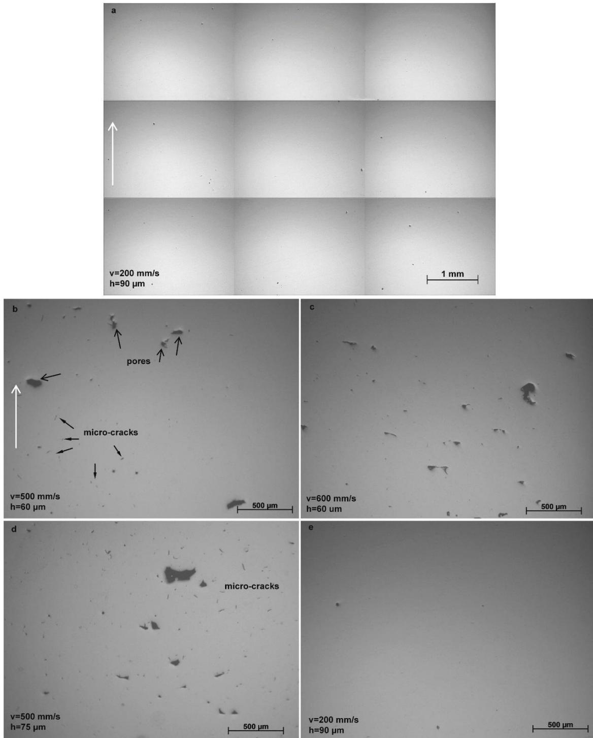
**Fig. 3.** OM images showing porosity and cracks in the vertical sections under different conditions: (a) elongated sample at 200mm/s, 90 μm; (b) 500 mm/s, 60 μm; (c) 600 mm/s, 60 μm; (d) 500 mm/s, 75 μm and (e) 200 mm/s, 90 μm; the white arrow indicates the building direction.
