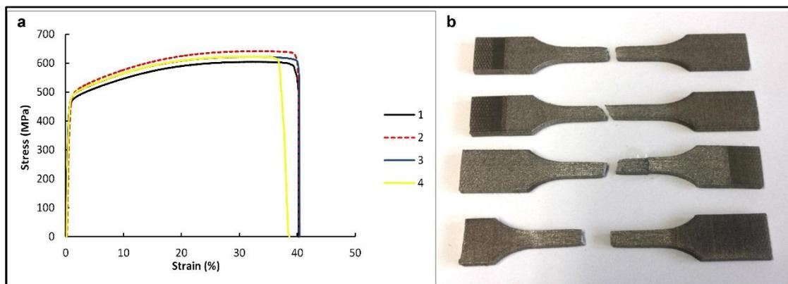
**Fig. 9.** Tensile performance of the as-fabricated Hastelloy-X samples.
