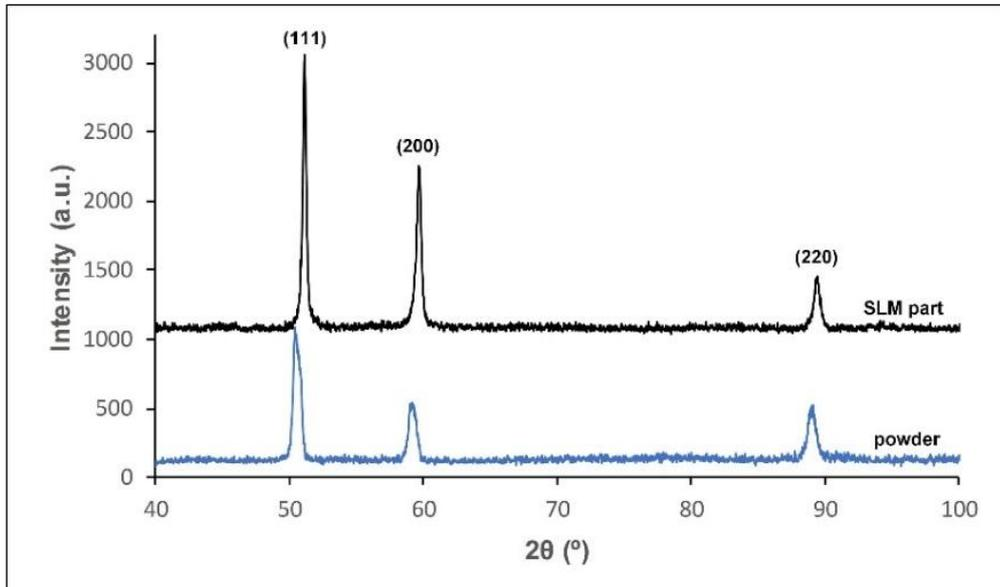
**Fig. 4.** XRD patterns of the Hastelloy-X powder and SLM-fabricated part.
