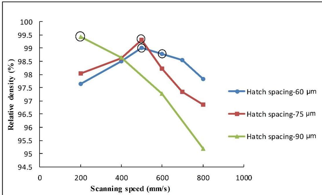
**Fig.2.** Relative density of the as-fabricated samples.
