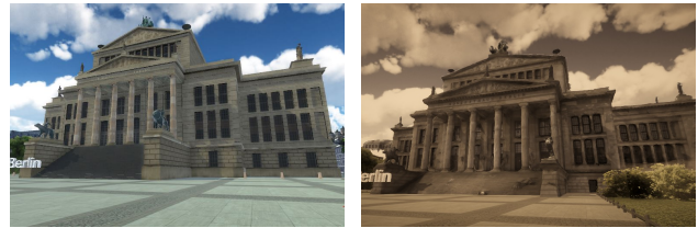
Figure 9: Comparison between manually a modeled concert house (left) and the result from 3D reconstruction (right) in the VR environment. There is a clear difference in length proportions.
