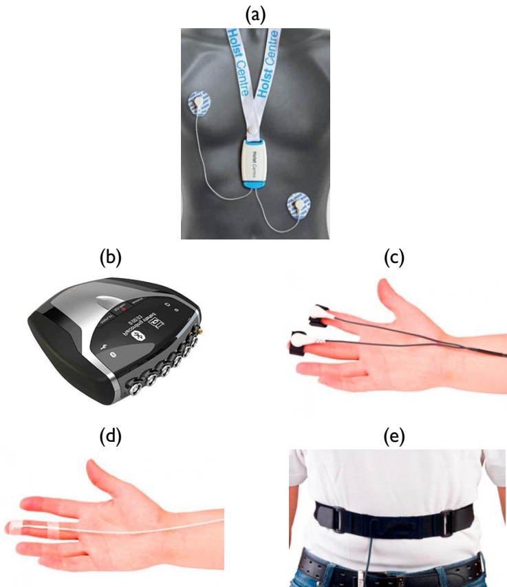
Figure 3-2: Necklace (a) for ECG recording and NeXus 10 – MK II (b-e) for SC, ST and respiration recordings
