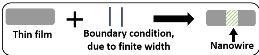
Figure 5.12 Schematic representation of a (rectangular) nanowire as though to be a thin film with an additional boundary condition (due to finite width)
