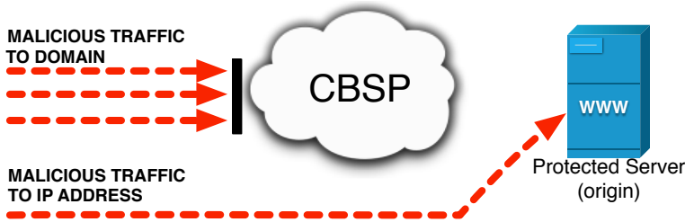
Figure 6.2: Bypassing cloud-based security. In the case of DNS rerouting, only traffic that uses the domain name is diverted through the CBSP’s network. Traffic that uses the IP address of the protected server can reach the web server directly.
