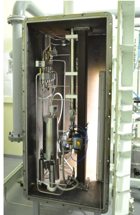
Fluid Hammer Facility (Chamber opened)
