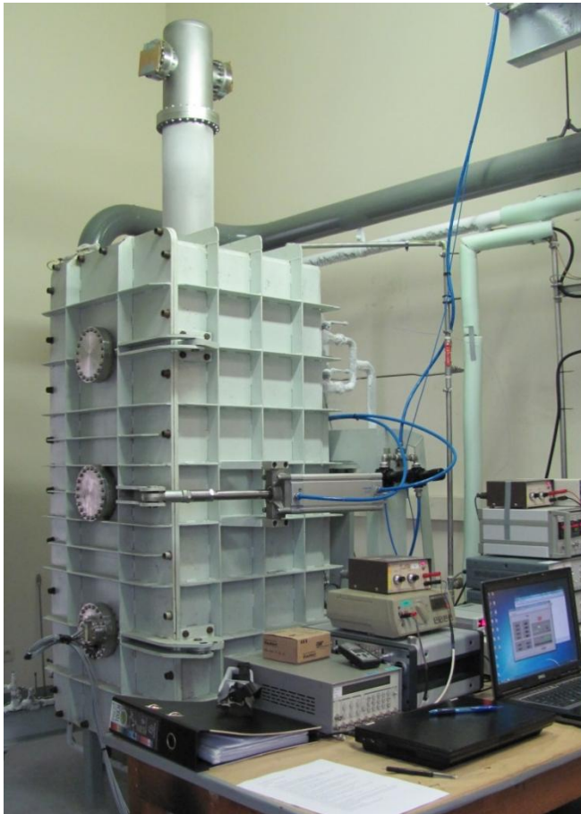
Fluid Hammer Facility (Chamber closed)
