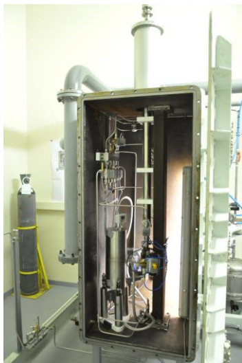
Figure 3. Cryogenic facility inside the vacuum chamber
