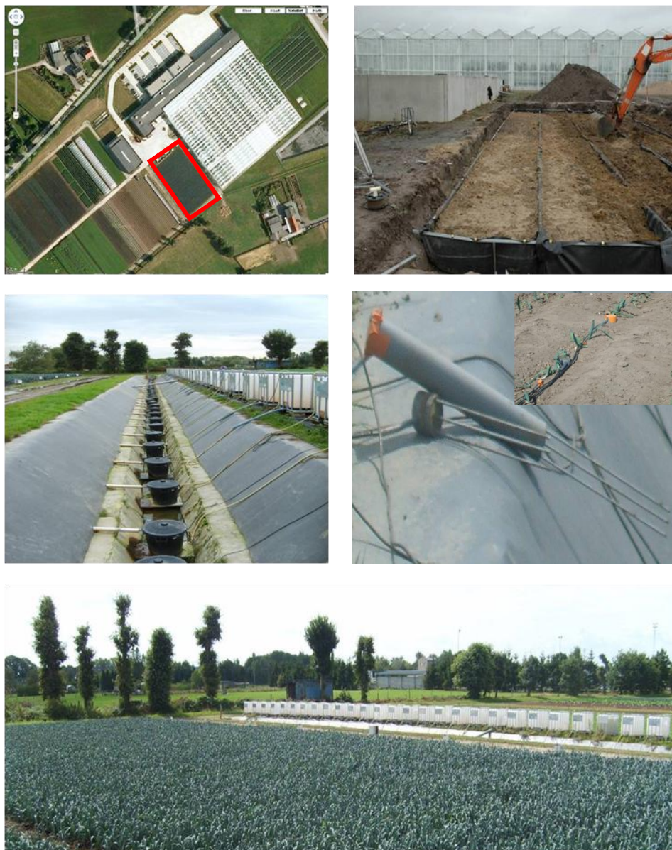
Figure 2-1 Overview of the experimental setup. From top to bottom, from left to right: i) aerial view of the Experimental station in Sint-Katelijne-Waver, Flanders and the experimental field (red square), ii) each subplot is contained in an impermeable foil, iii) collection of leaching water, iv) soil moisture and temperature sensors, and v) the experimental field, covered by leek.
