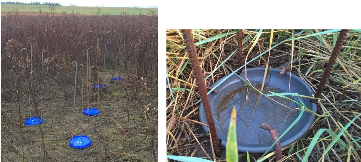
**Figure S3-2** Pictures of the sediment traps used to collect sediments deposited on the tidal marsh during inundation events. The blue lid floats on the water when the marsh is inundated, so that sediments are deposited in the grey tray (right picture). After inundation, the blue lid drop on the tray, to prevent contamination of deposited sediments and loss of sediment due to potential raindrop impact (left picture).
