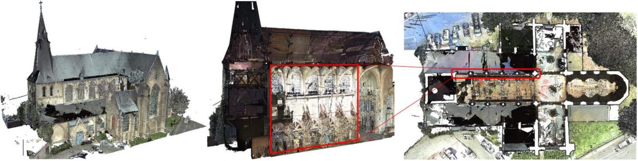
**Figure 1.** Overview point cloud data Sint-Jacobs Church, Leuven, Belgium: Colorized point cloud (left), Elevation view with northern nave wall in red (mid) and plan view northern nave wall in red (right).
