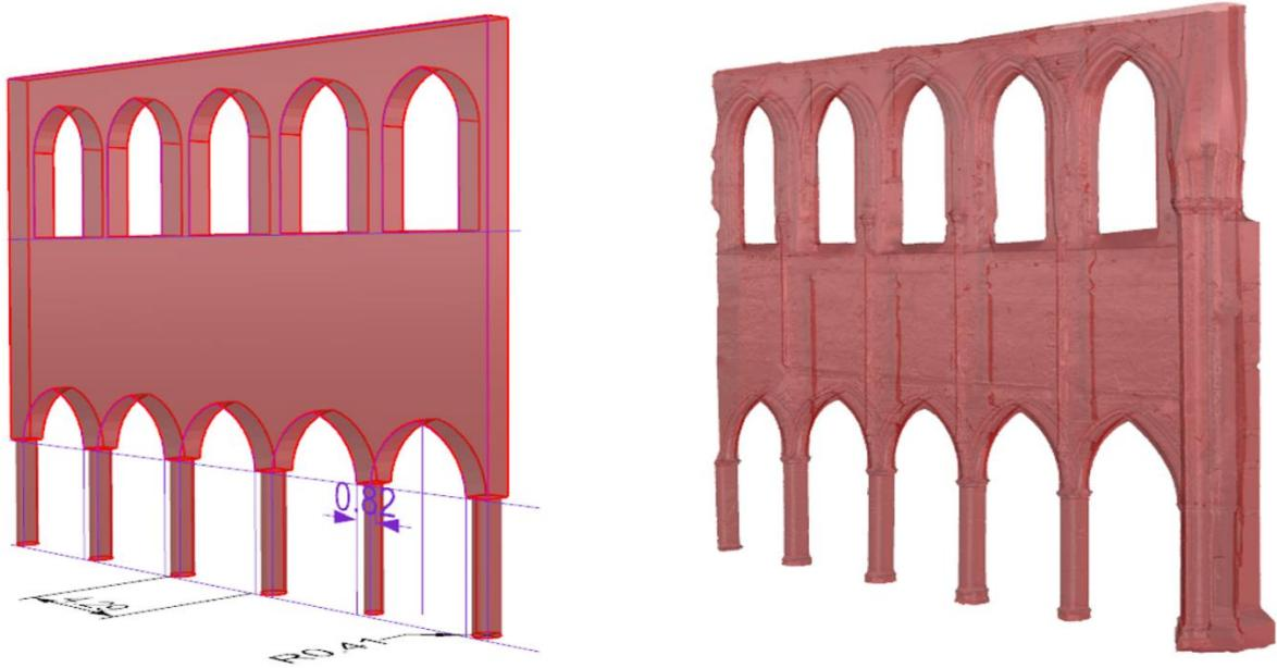
**Figure 5.** Overview of the traditional wire-frame FEM mesh (left) and the automatically reconstructed FEM Mesh from point cloud data (right).
