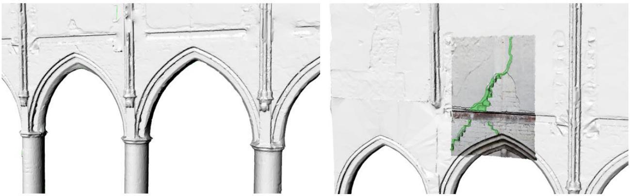
**Figure 7.** Complexity of arches FEM mesh near the connection of the walls and the columns (Left) and modelled cracks in FEM (right).
