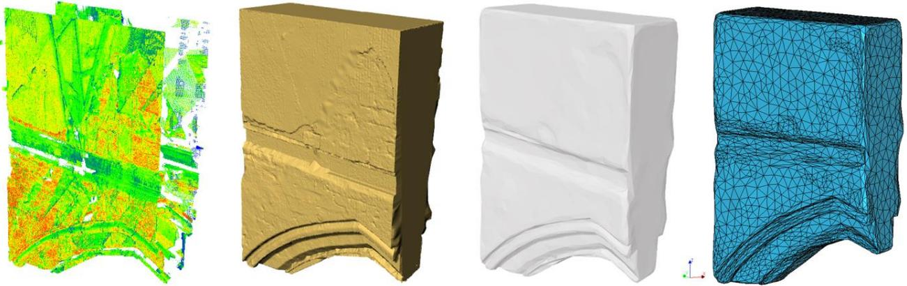
**Figure 2.** Overview methodology FEM mesh creation: Point cloud colored by intensity (a), Watertight triangular mesh (b), Volumetric simplified mesh (c) and final FEM mesh (d).
