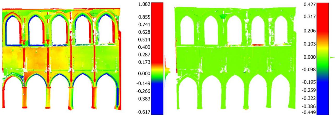
**Figure 6.** Signed distance [m] between the point cloud and the traditional wire-frame FEM Mesh (left) and FEM complex mesh (right).
