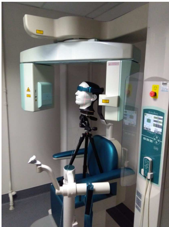
Figure 7.8: Phantom study setup. An anthropomorphic phantom was positioned at the center of the scanner FOV.
