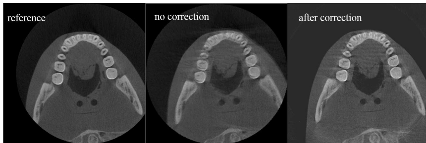
Figure 7.9: Left is a 2D transaxial plane in the reference image. Middle is the same plane in the uncorrected image. Right is the same plane in the corrected image, where artifacts are much less than the middle one. Note that we have also performed our own reconstruction for the static scan (not shown), and the resulted image looks quite similar to the machine reconstruction.
